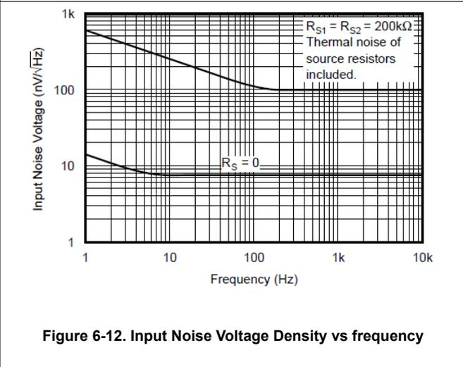
Figure 6-12. Input Noise Voltage Density vs frequency
