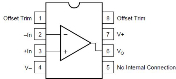
**Figure 5-1. D Package, 8-Pin SOIC
