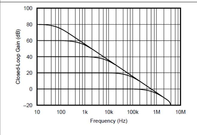
Figure 6-6. Closed-Loop Response vs Frequency
