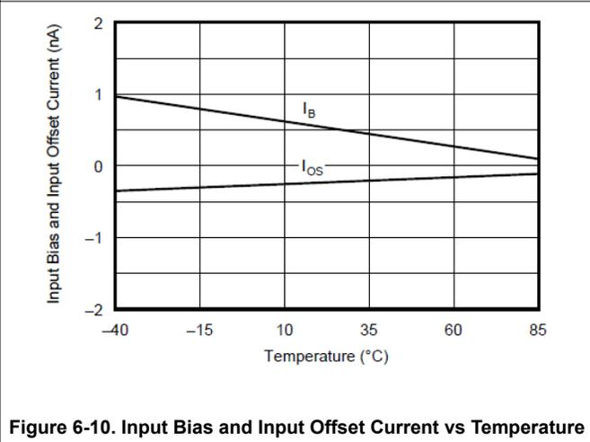
Figure 6-10. Input Bias and Input Offset Current vs Temperature
