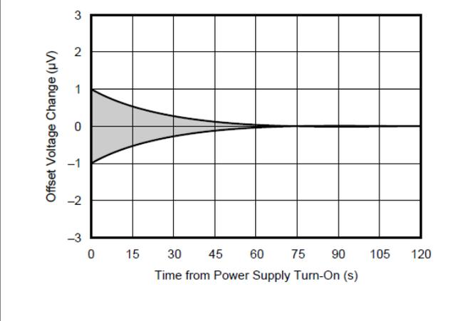
Figure 6-4. Warm-Up Offset Voltage Drift
