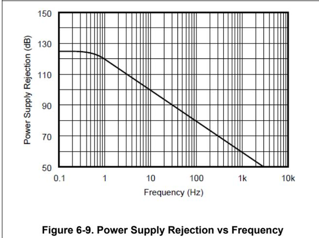
Figure 6-9. Power Supply Rejection vs Frequency
