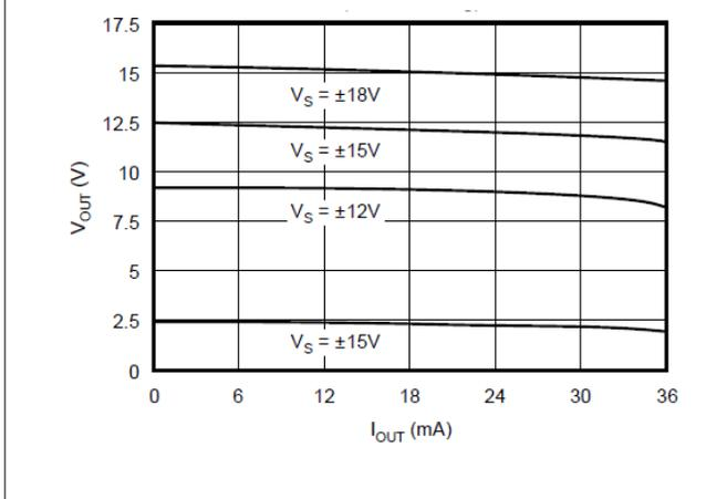
Figure 6-3. Maximum  $V_{OUT}$  vs  $I_{OUT}$  (Positive Swing)
