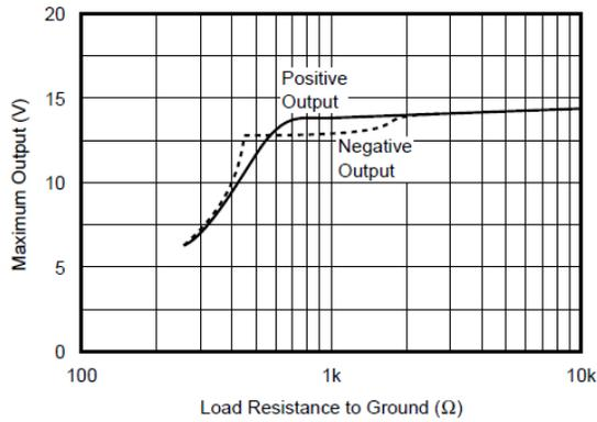
Figure 6-15. Maximum Output Voltage vs Load Resistance
