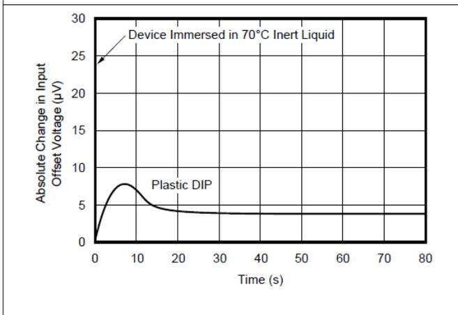
Figure 6-5. Offset Voltage Change Due To Thermal Shock
