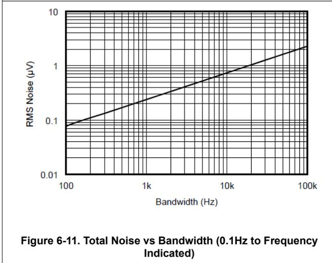
Figure 6-11. Total Noise vs Bandwidth (0.1Hz to Frequency Indicated)
