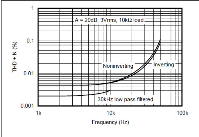
Figure 6-1. Total Harmonic Distortion and Noise vs Frequency
