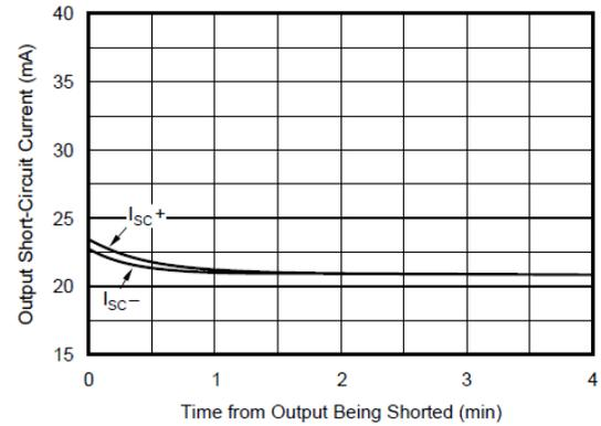
Figure 6-16. Output Short-Circuit Current vs Time
