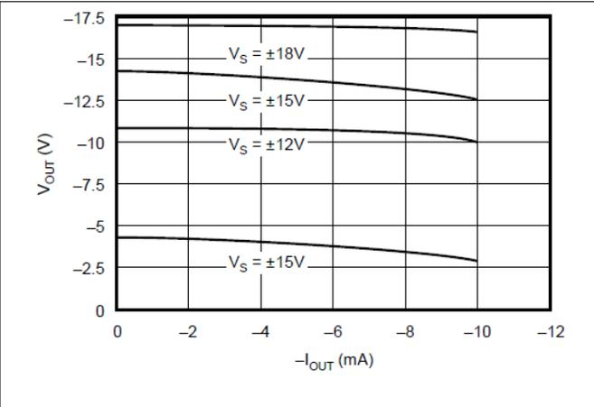
Figure 6-2. Maximum  $V_{OUT}$  vs  $I_{OUT}$  (Negative Swing)
