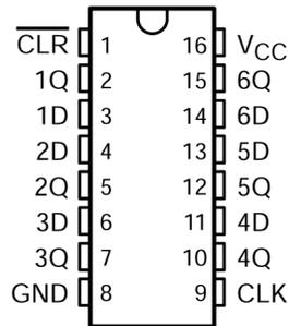
Figure 4-1. D or N Package (Top View)
