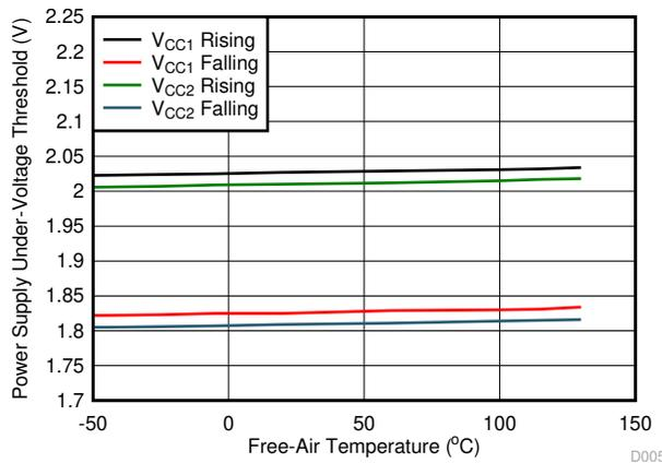
**Figure 5-9. Power Supply Undervoltage Threshold vs Free-Air Temperature**
