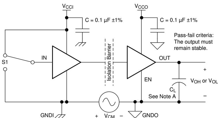
A. C<sub>L</sub> = 15pF and includes instrumentation and fixture capacitance within ±20%.
