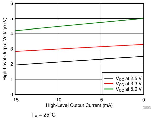
**Figure 5-7. High-Level Output Voltage vs High-level Output Current**
