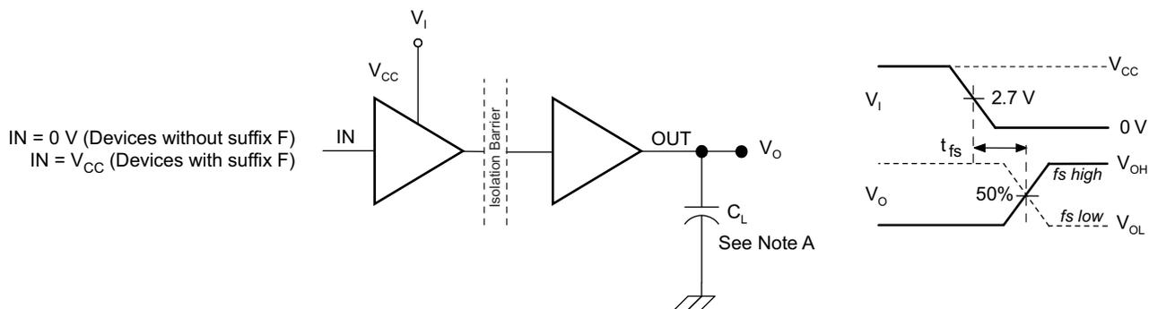
A. C<sub>L</sub> = 15pF and includes instrumentation and fixture capacitance within ±20%.
