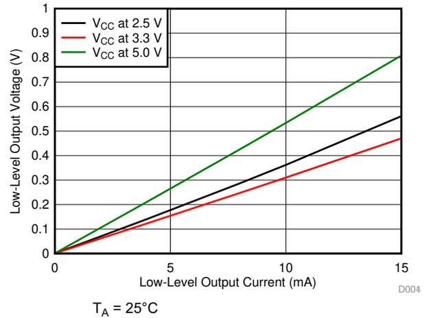
**Figure 5-8. Low-Level Output Voltage vs Low-Level Output Current**
