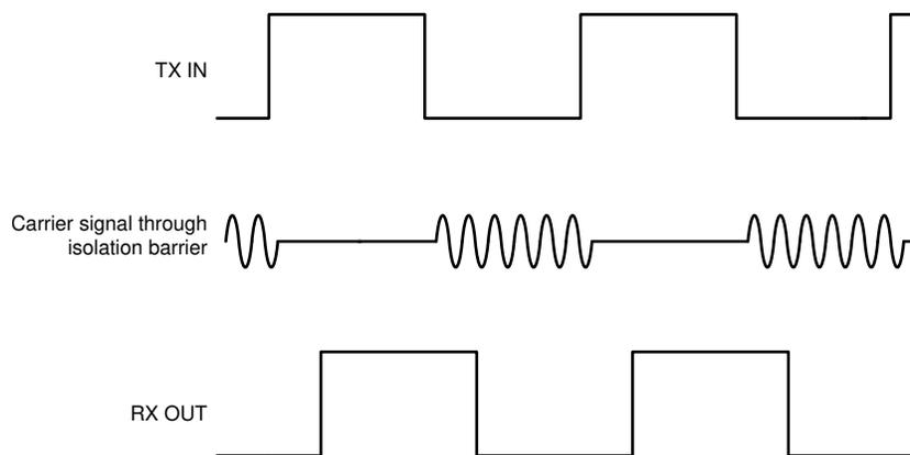
**Figure 6-2. On-Off Keying (OOK) Based Modulation Scheme**
