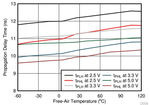
**Figure 5-10. Propagation Delay Time vs Free-Air Temperature**
