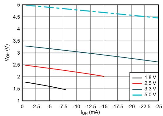
**Figure 6-4. Output Voltage vs Current in HIGH State**
