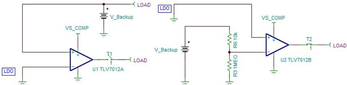
5. Set the voltage divider created by  $R_3$  and  $R_6$  for a ratio of 1%. Set the ratio for 1% so that U2 can quickly switch once the LDO loses power. During normal operation, OUT\_BU will stay high because the inverting input will be 1% less than inverting input. When the main supply loses power, OUT\_BU will go high because the non-inverting input is connected to the output of the LDO.
