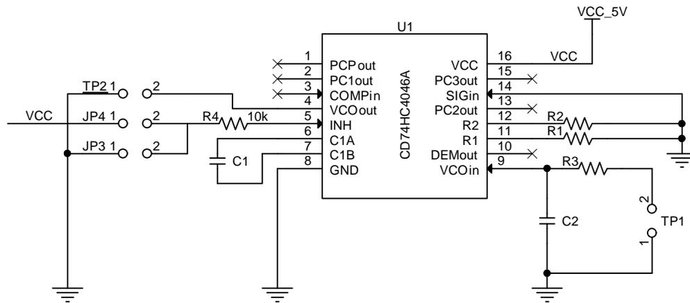
Figure 4. Typical Modulator Schematic
