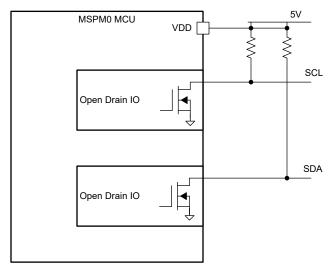
Figure 1-1. Subsystem Functional Block Diagram
