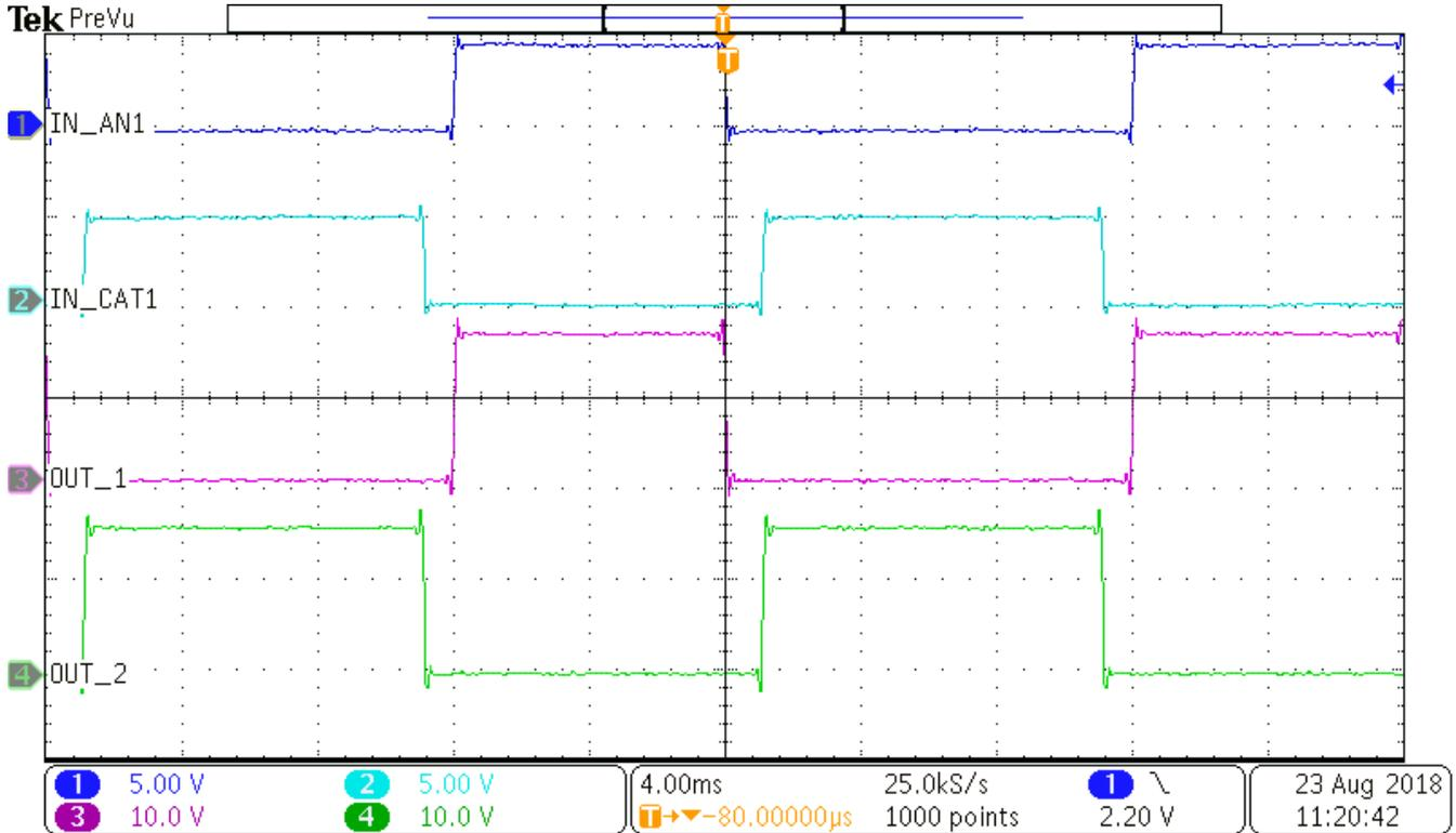
Figure 5. Interlock Functionality
