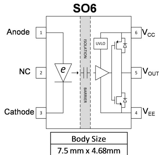
**Figure 1. UCC23513 Pinout**
