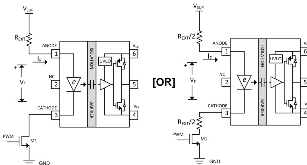
Figure 2. Input Drive with NMOS at Cathode
