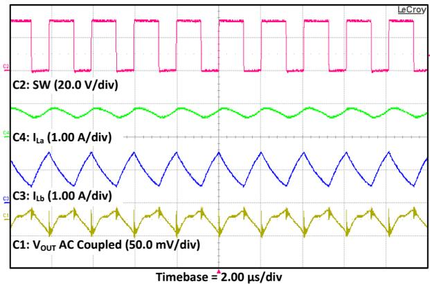
Figure 8. Current Ripple With 20 µF  $C_P$
