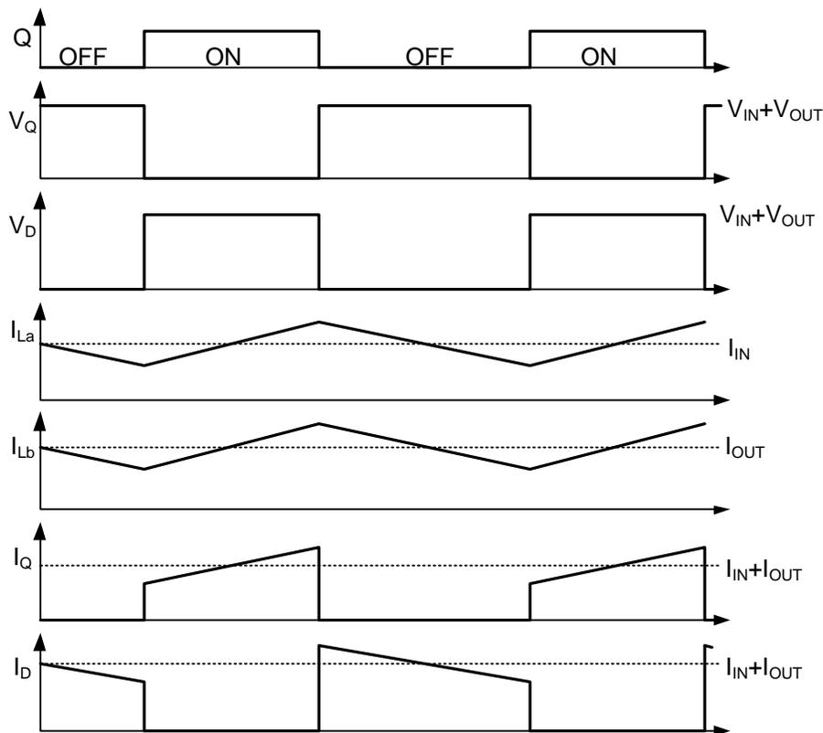
**Figure 3. Voltage and Current Waveforms in a SEPIC**
