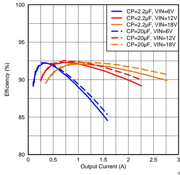
Figure 9. CCM Efficiency Using 2.2 µF and 20 µF  $C_p$
