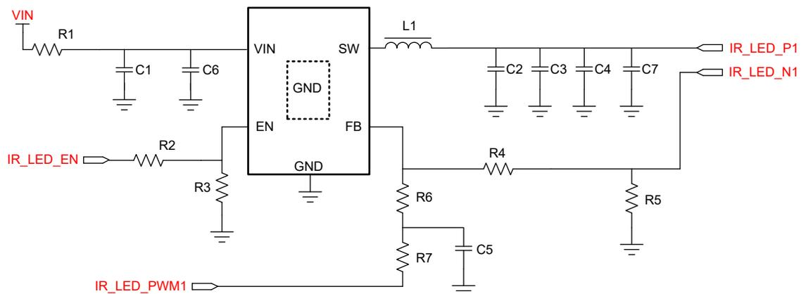
**Figure 3-2. Design Schematic**
