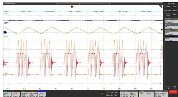
Figure 4-8. Output Current Ripple of TPS92201A at Light Load
