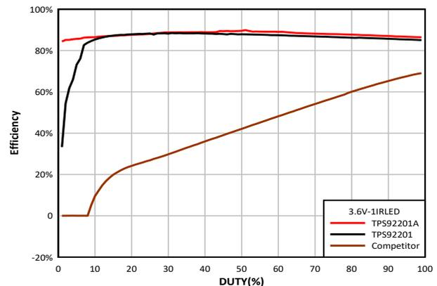
Figure 4-3. Efficiency\_1IR\_3.6V
