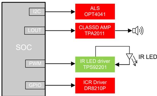
Figure 1-1. Simply Block Diagram in IR LED system
