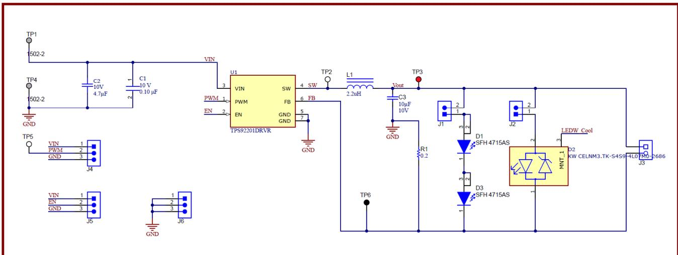
Figure 1-3. TPS92201 EVM Schematic
