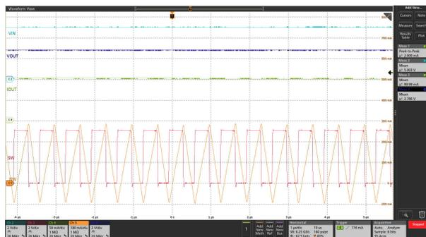
Figure 4-7. Output Current Ripple of TPS92201 at Light Load
