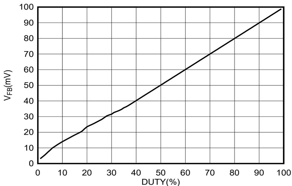
Figure 2-1. DIM Duty Cycle vs FB Voltage in Analog Dimming
