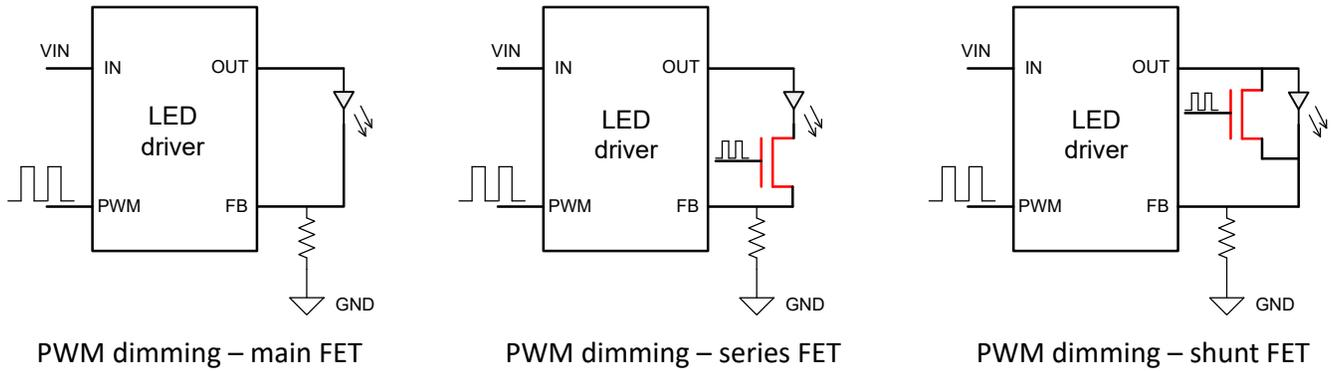
**Figure 2-2. Three Types of PWM Dimming**
