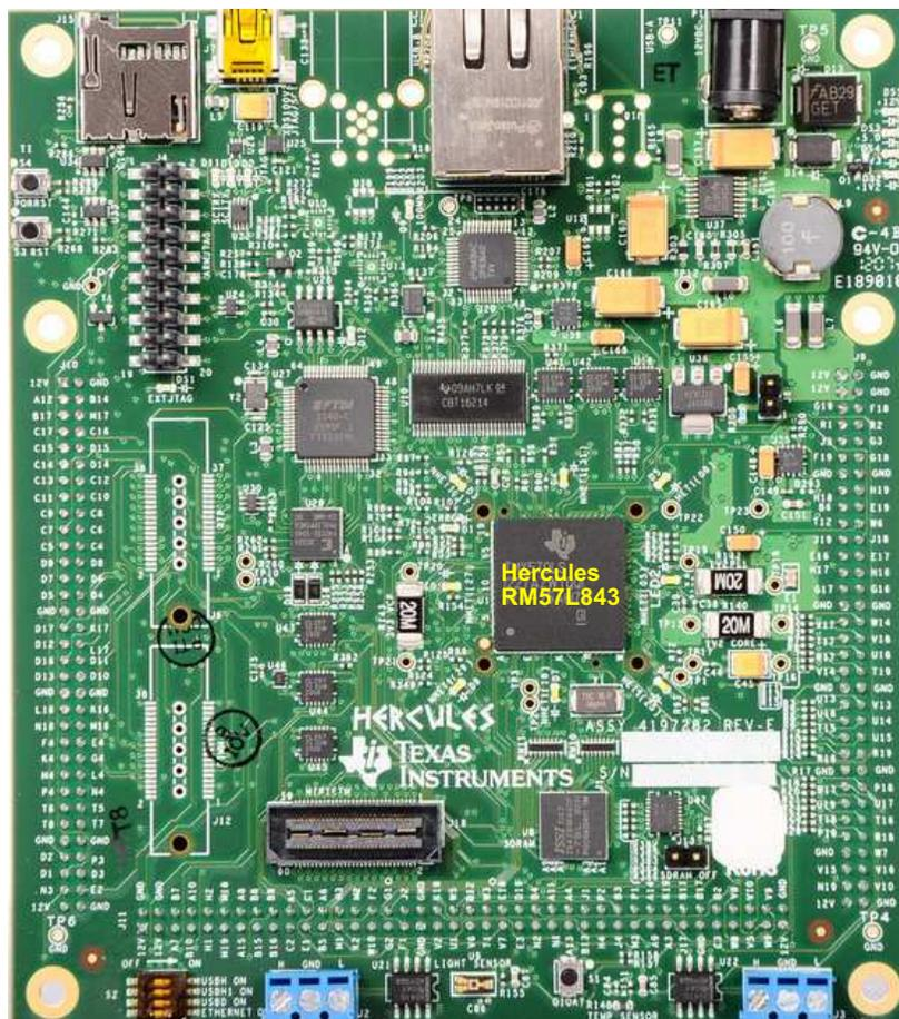
Figure 2-1. RM57L HDK Board, Interfaces Top Side
