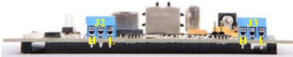
Figure 2-4. J2, J3 CAN Bus Interface (Screw Terminal)
