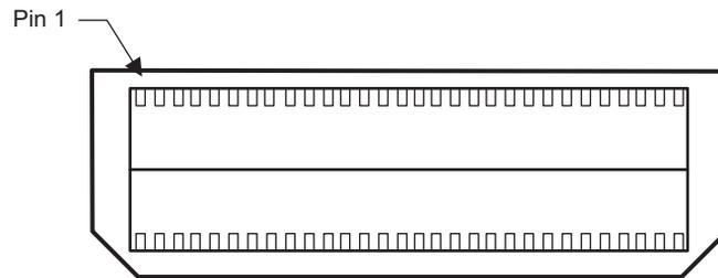
**Figure 2-5. J19, 60 Pin MIPI ETM Header**
