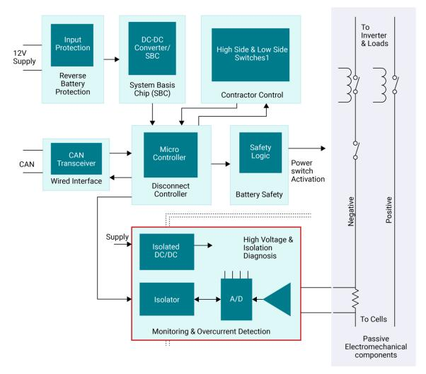
Figure 1. Battery disconnect unit system block diagram
