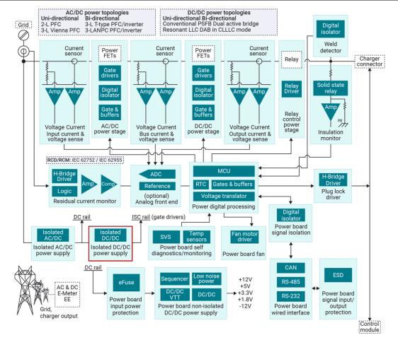
Figure 2. EV charging station system block diagram
