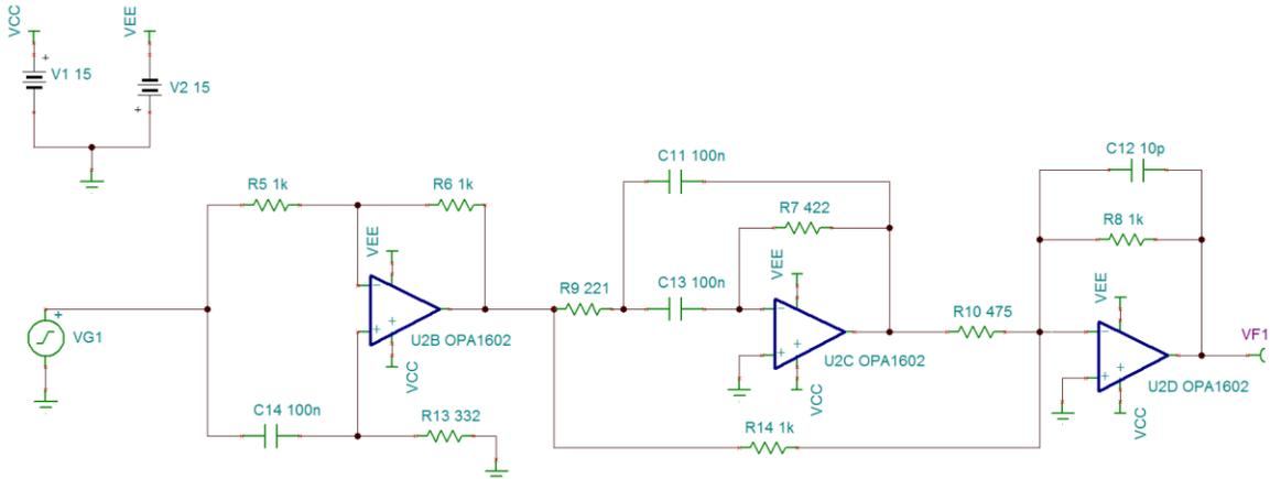
**Figure 30: Tina-TI™ simulation schematic for testing all-pass filter delay.**
