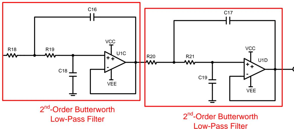
Figure 9: A 4th-Order Linkwitz-Riley low-pass filter made by cascading two 2<sup>nd</sup>-order Butterworth low-pass filters
