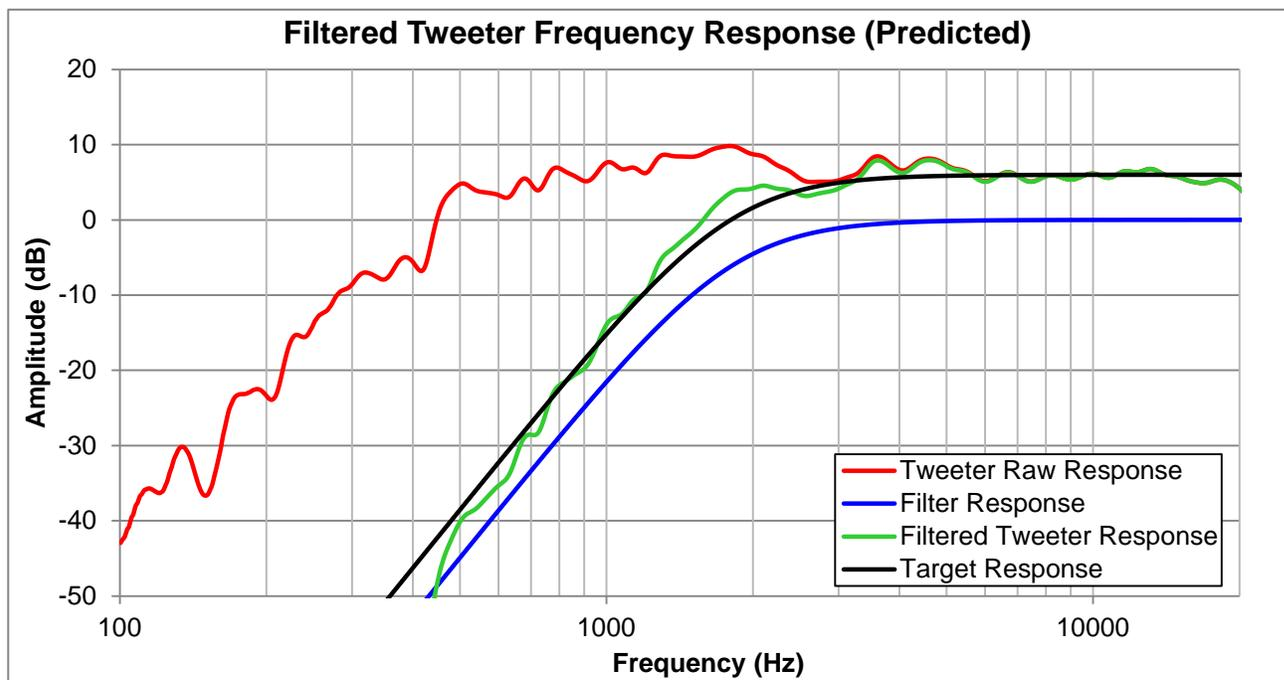
**Figure 15: Tweeter frequency response without filtering (red) and with a 1.8 kHz 4<sup>th</sup>-order Linkwitz-Riley high-pass filter (green). The filter response and target responses are shown in blue and black respectively**
