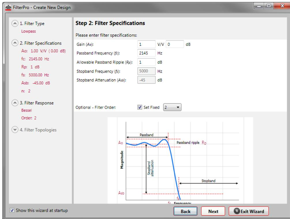
Figure 10: The Filter Specifications window of the FilterPro™ New Design Wizard
