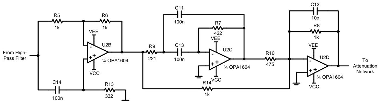
Figure 19: A 3rd-order all-pass filter providing 155 us delay to the tweeter signal path
