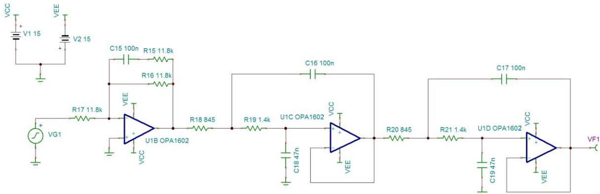
**Figure 24: Tina-TI™ simulation schematic of the woofer signal path**
