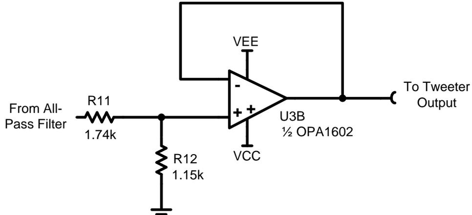
**Figure 21: Tweeter level correction and output buffer circuit.**
