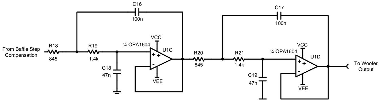
**Figure 14: Final 1.8 kHz, 4<sup>th</sup>-order Linkwitz-Riley low-pass filter**
