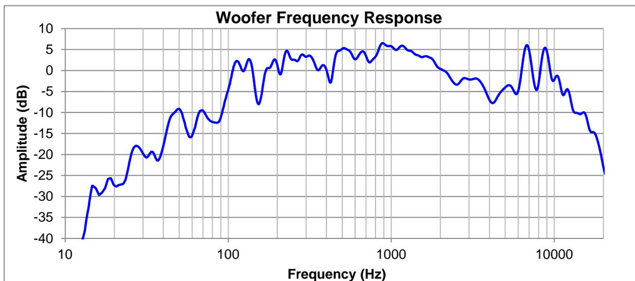
**Figure 3: Woofer frequency response measured at a 1m distance on the tweeter axis (designed listening position). 1/8<sup>th</sup> Octave smoothing is applied and no gating is used (includes room effects)**
