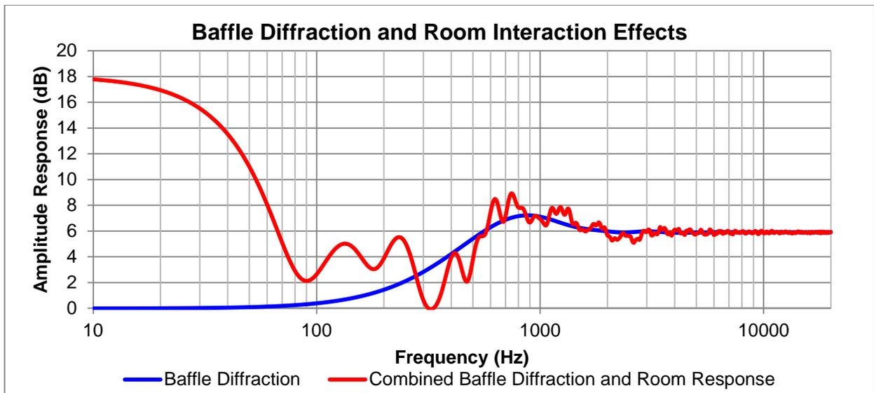
**Figure 4: Predicted baffle diffraction effects (blue curve) of a 178 mm woofer mounted on an 216 mm x 356 mm baffle (13 mm radius edge rounding). The center point of the woofer is 127 mm from the bottom edge. The red curve includes room acoustic effects as well. Curves generated by Baffle Diffraction and Boundary Simulator v1.2 © Jeff Bagby, used with permission.**
