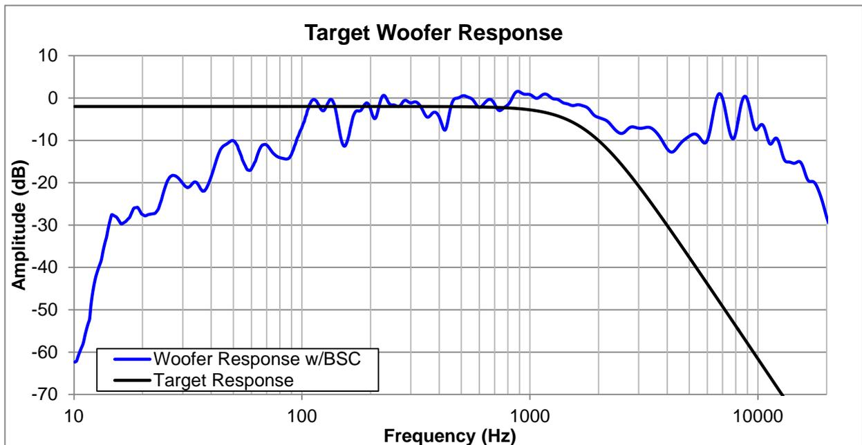
**Figure 7: Woofer frequency response including baffle step compensation (blue) and the target 4<sup>th</sup>-order Linkwitz-Riley low-pass transfer function with 1.8 kHz corner frequency (black)**
