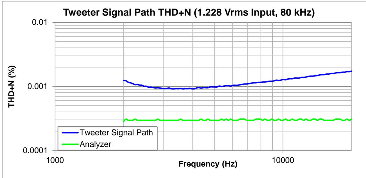
Figure 36: Measured THD+N of the tweeter signal path.
