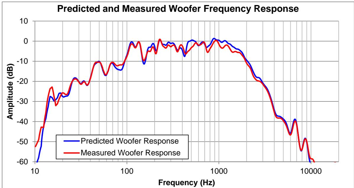
**Figure 38: Predicted and measured acoustic transfer function of the woofer. 1/8th octave smoothing**
