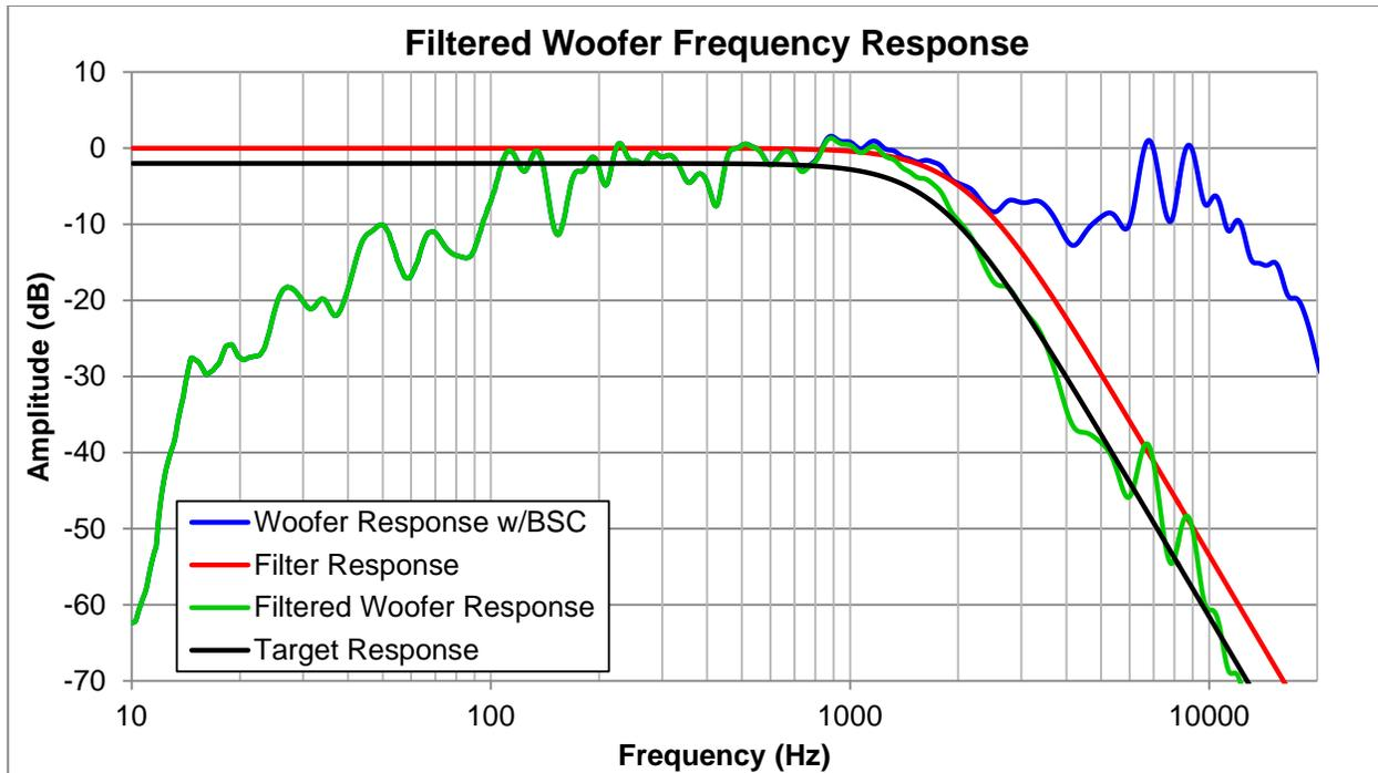
Figure 8: The woofer's frequency response including the filter response (green). The filter frequency response is shown in red, target response in black, and woofer response with baffle step compensation (BSC) shown in blue
