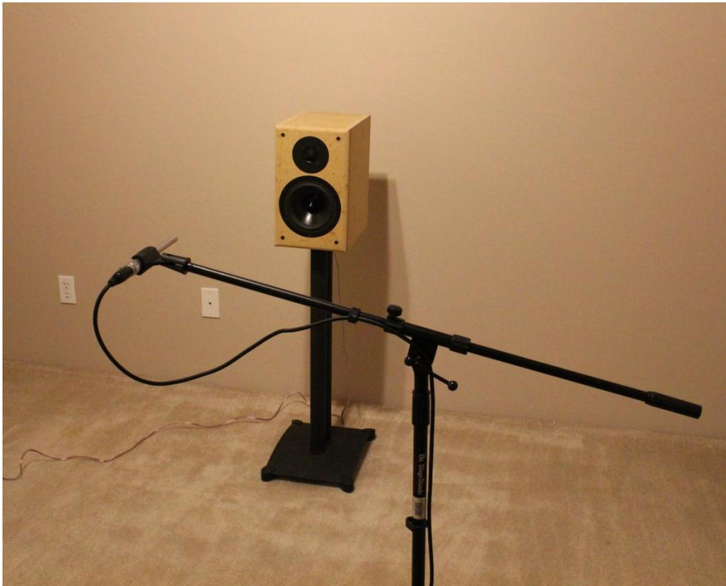
**Figure 43: The loudspeaker under test with a calibrated measurement microphone placed on the tweeter axis at a 1 m distance.**
