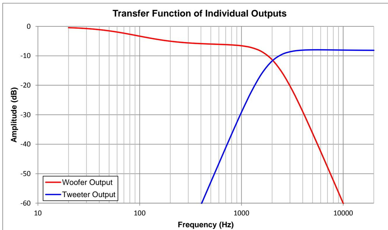
**Figure 1: Measured Transfer Function of the crossover network.**
