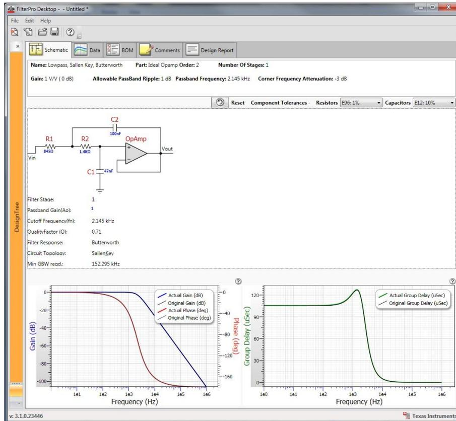
**Figure 13: Final 2<sup>nd</sup>-order Butterworth low-pass filter design using 1% resistor tolerances and 10% capacitor tolerances. The value for C2 was forced to 100nF**
