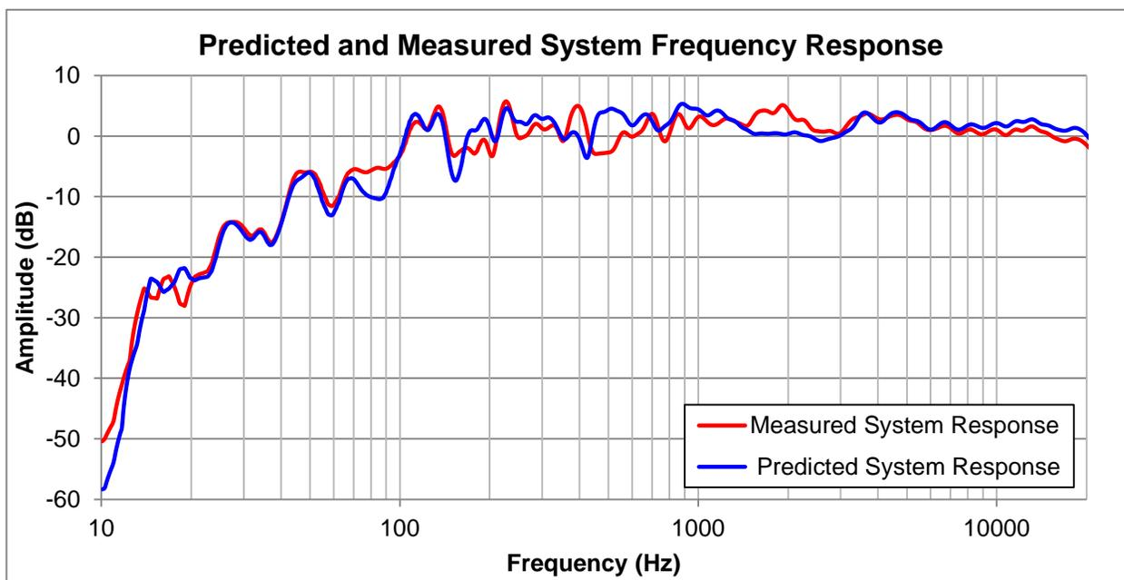
Figure 40: Predicted and measured system frequency response.
