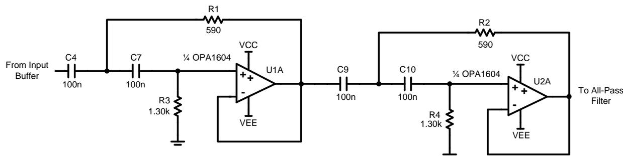
**Figure 16: 4<sup>th</sup>-order Linkwitz-Riley high-pass filter in the tweeter signal path**
