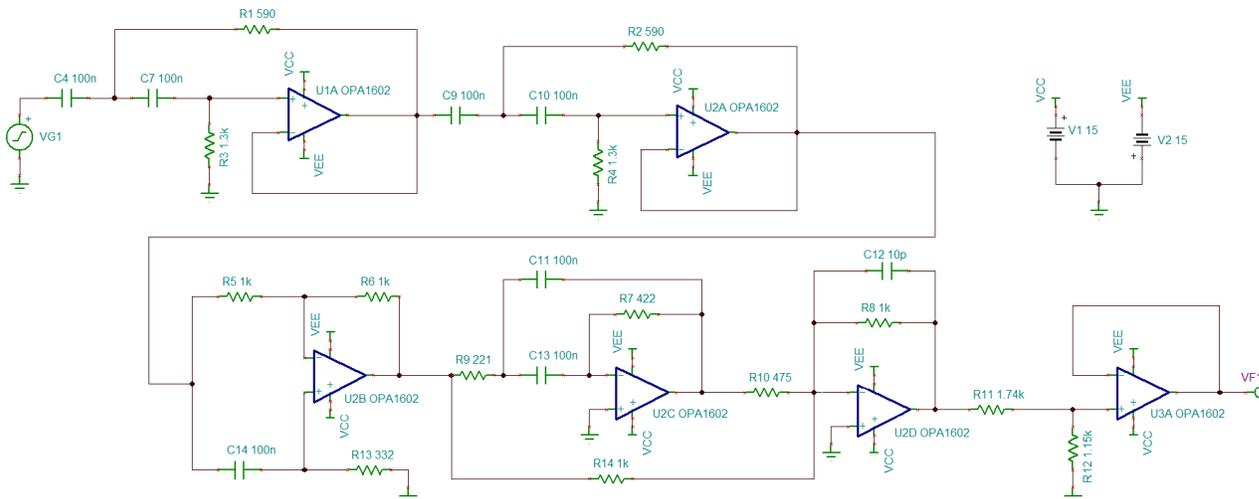
Figure 27: TINA-TI™ simulation schematic of the tweeter signal path.
