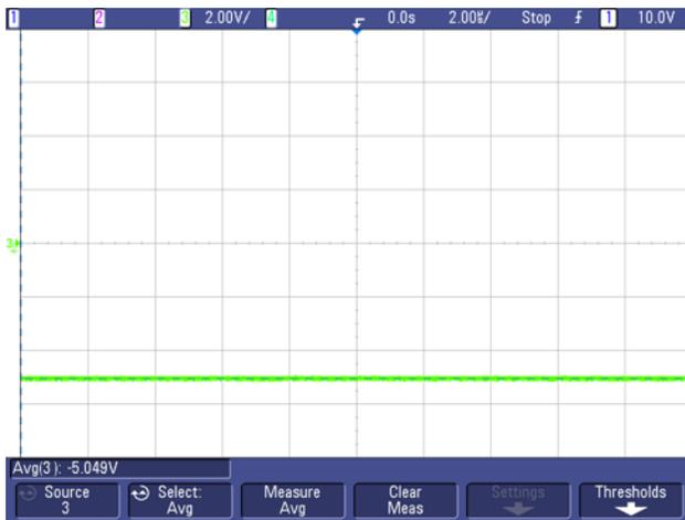
Figure 92.  $V_{OUT} = -5\text{ V}$  at  $V_{IN} = 24\text{ V}$
