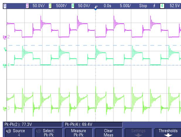
**Figure 60. MOSFET Stress VDS for –HV Output**
