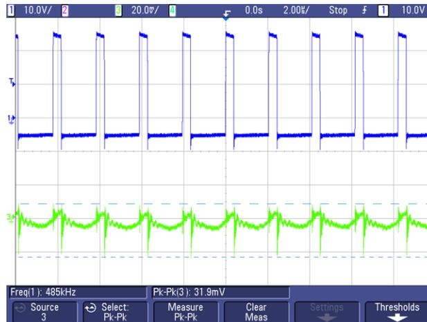
Figure 94. SW Node Waveform and Output Ripple for  $V_{OUT} = -5\text{ V}$ ,  $I_{OUT} = -1\text{ A}$
