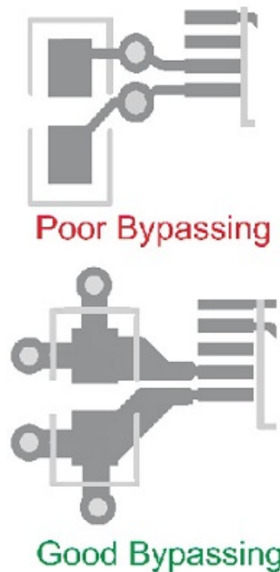
Figure 3. Decoupling Capacitor Example
