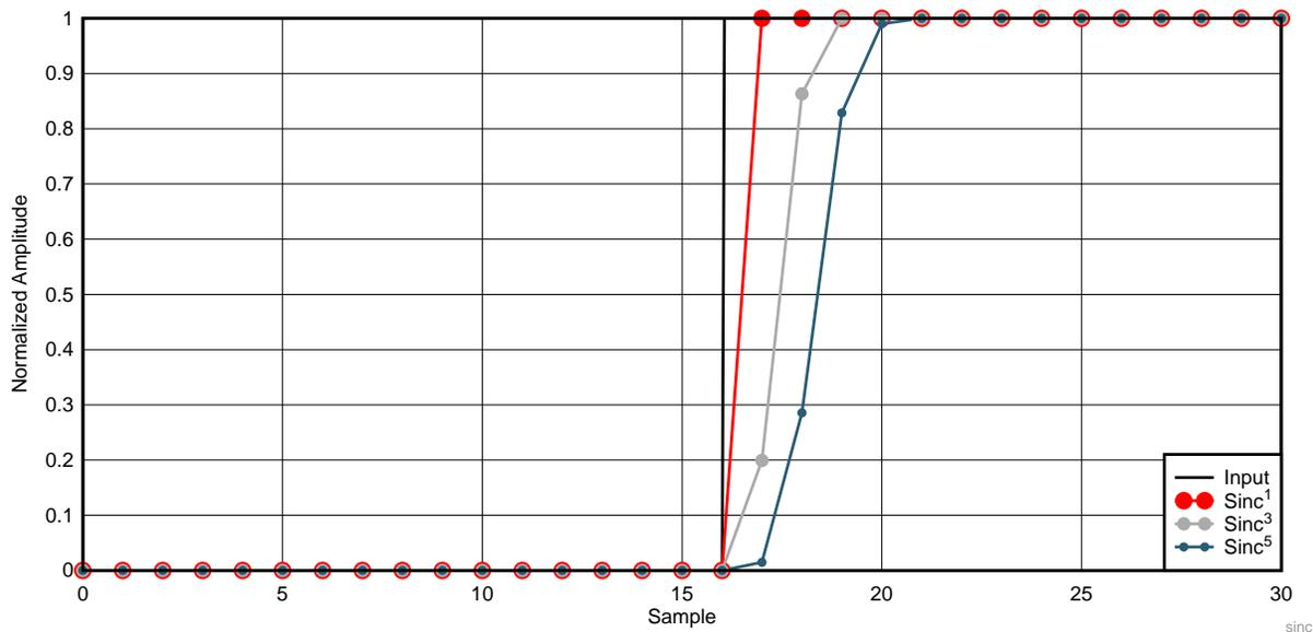
Figure 5. Step Response for Sinc<sup>1</sup>, Sinc<sup>3</sup>, and Sinc<sup>5</sup> Digital Filters
