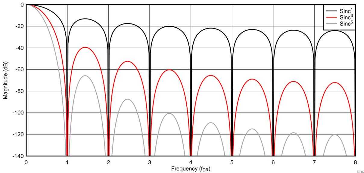
Figure 4. Frequency Response of Sinc<sup>1</sup>, Sinc<sup>3</sup>, and Sinc<sup>5</sup> Digital Filters
