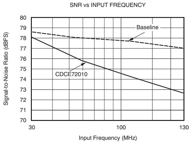
**Figure 11. SNR Performance vs IF Input Frequency**
