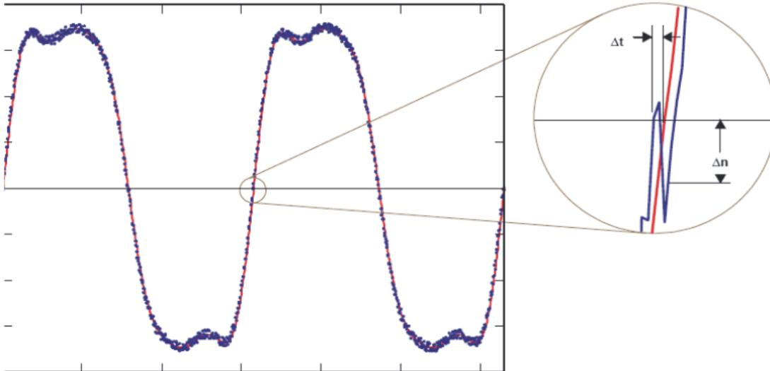
Figure 4. Sampling Error Caused by Thermal Noise Component
