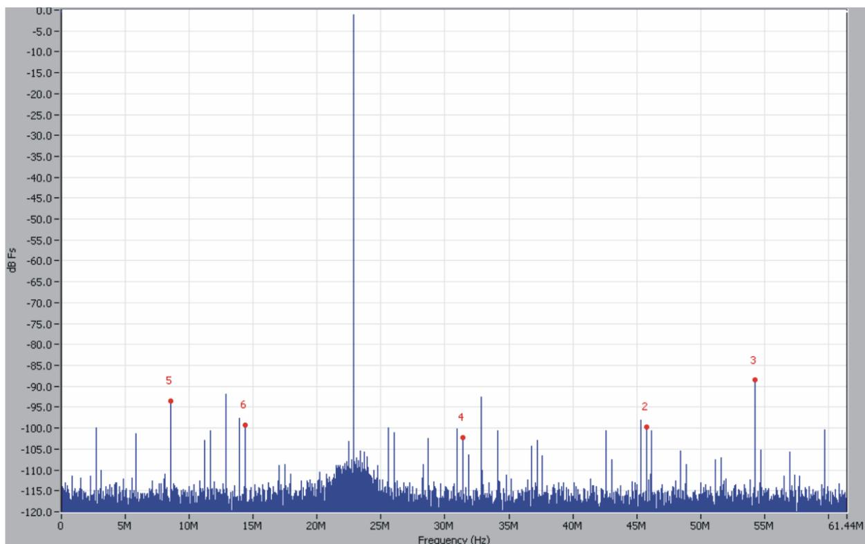
Figure 16. Spectral Performance with the CDCE72010-BPF-Transformer at 100-MHz IF Input
