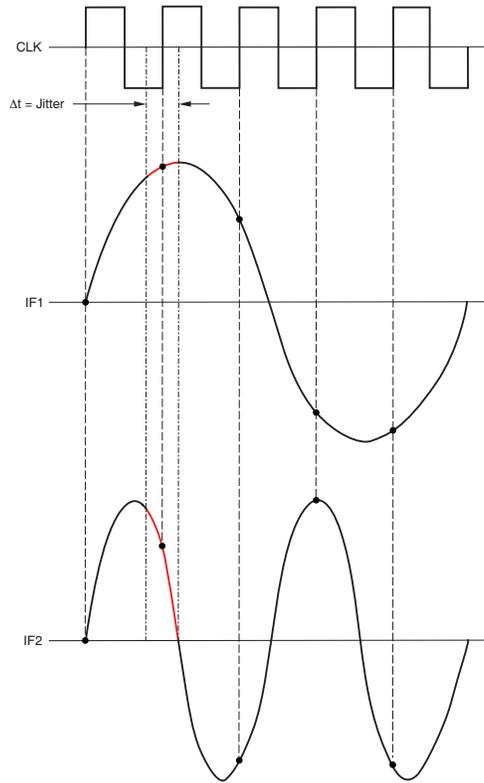
**Figure 2. SNR Degradation as a Result of Jitter for Different IF Input Signals**
