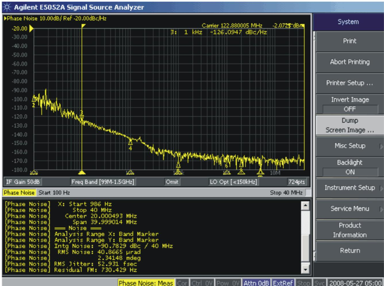
Figure 14. CDCE72010 122.88-MHz Filtered LVCMOS Output Phase Noise
