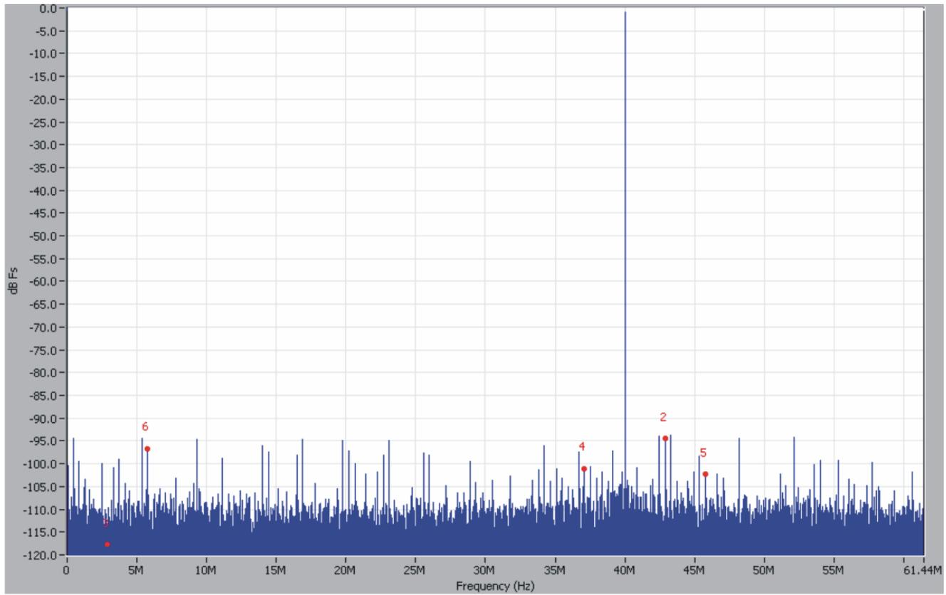
**Figure 12. Spectral Performance with the CDCE72010 Clock Source at 30-MHz IF Input**
