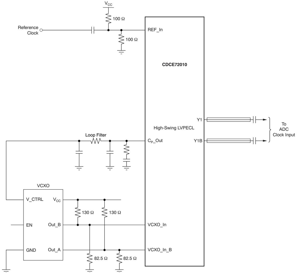
**Figure 7. CDCE72010 Interface to ADCs for Low-/Mid-IF Input Frequencies**
