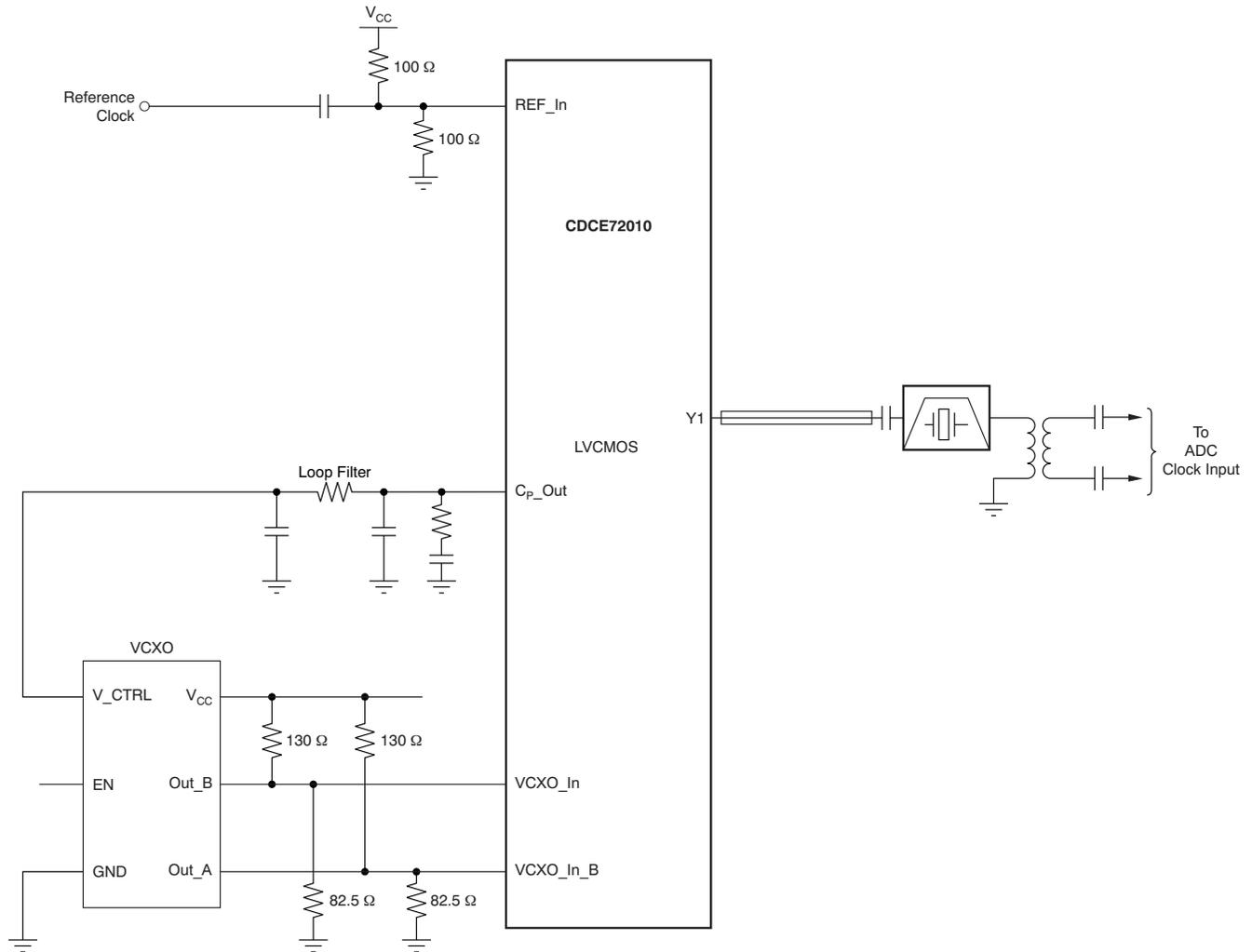
Figure 8. CDCE72010 Interface to ADCs for High-IF Input Frequencies
