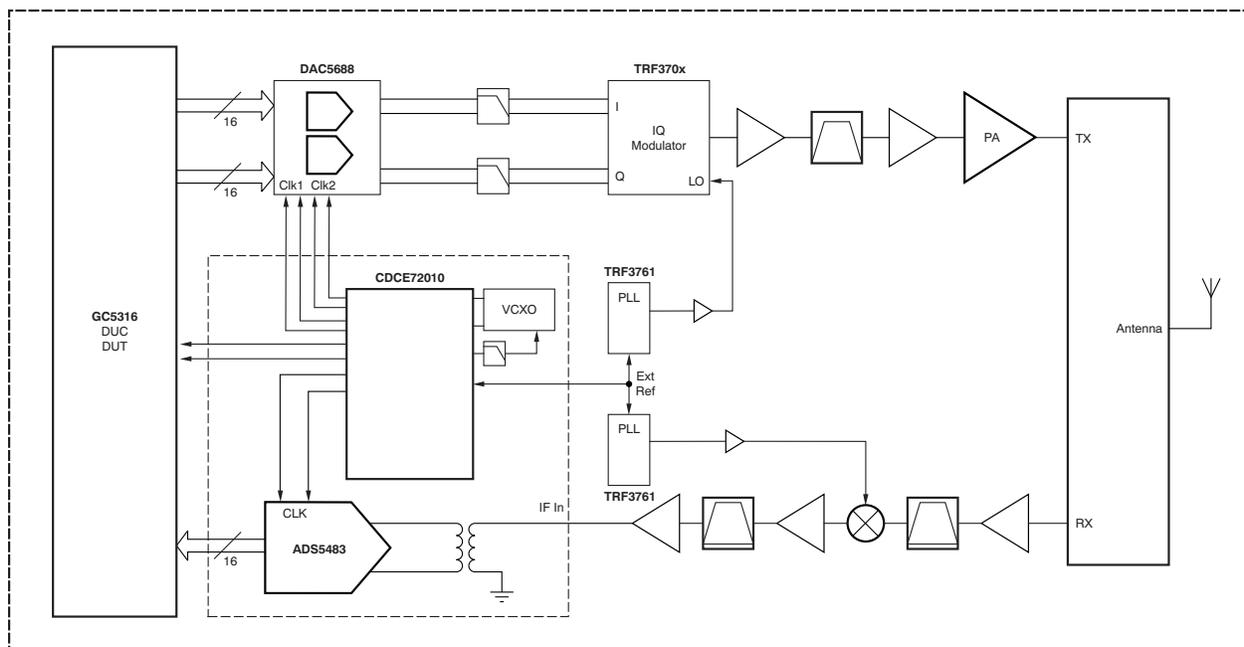
**Figure 1. ADS5483 ADC with the CDCE72010 Clocking Solution Within a Typical Base Station Architecture**
