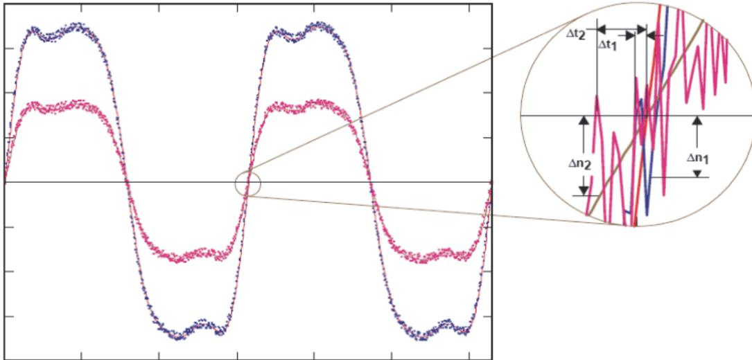
**Figure 5. Thermal Noise Effect for Different Slope Clock Signals**
