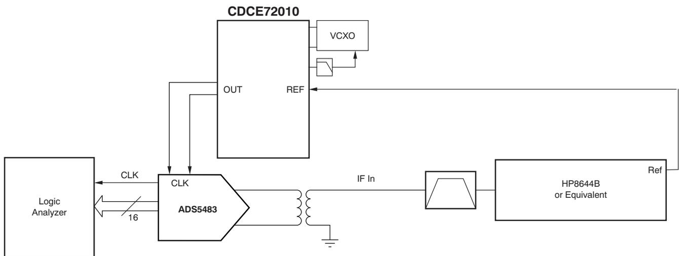
**Figure 10. ADC Evaluation Test Setup with the CDCE72010 as Clock Source**
