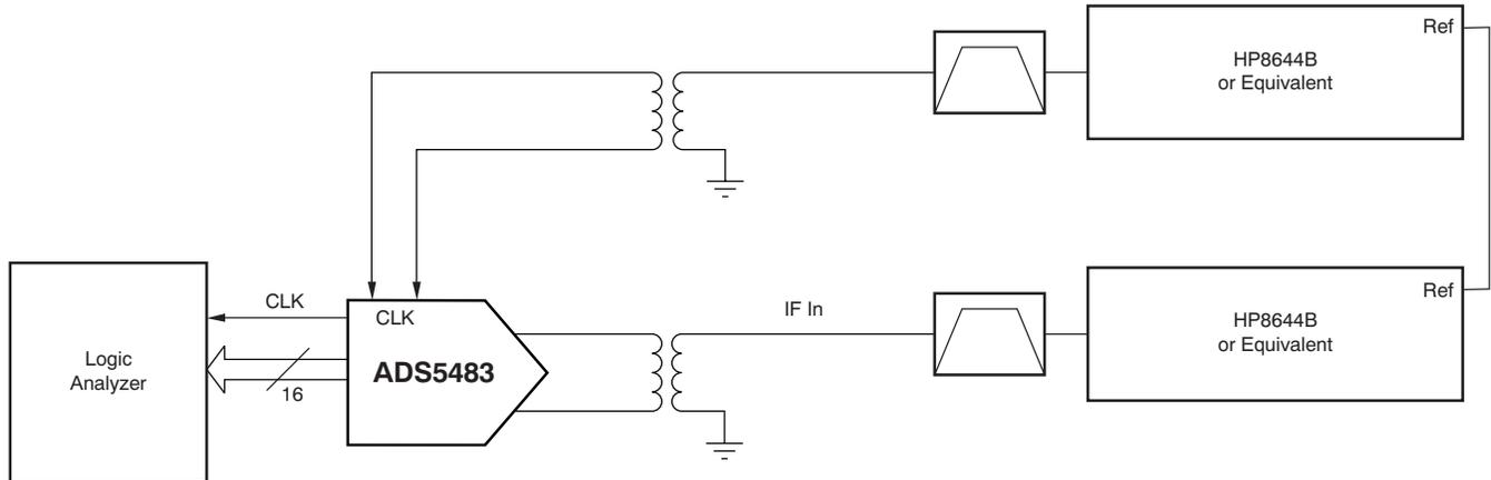
**Figure 9. ADC Evaluation Test Setup (Baseline)**
