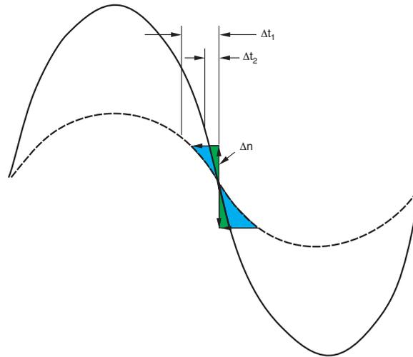
**Figure 6. Thermal Noise Effect for Different Amplitude Sinusoids**
