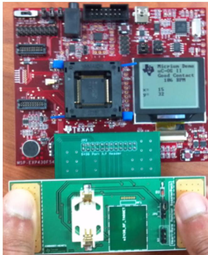
**Figure 1. MSP-EXP430F5438 With HRM BoosterPack Hardware Setup**
