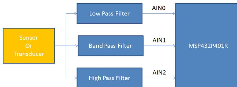
**Figure 3. Hardware Architecture**
