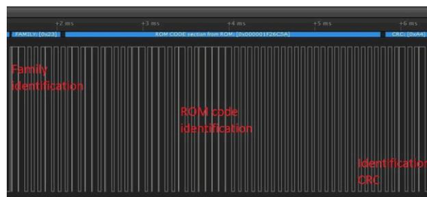
Figure 3. Single-Wire Reception of 64-bit Identification Number
