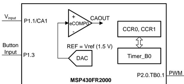
Figure 1. eCOMP ADC And PWM Output Block Diagram
