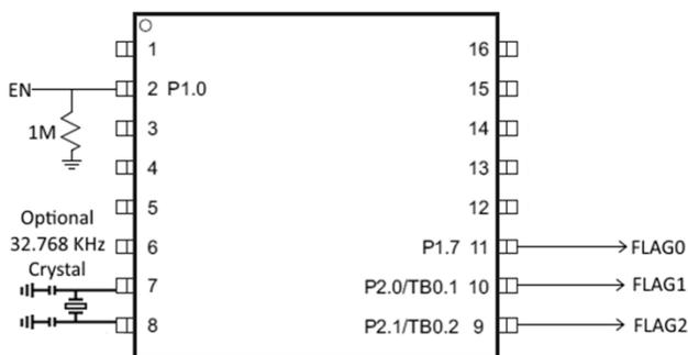
**Figure 1. Power Sequencer Inputs and Outputs**
