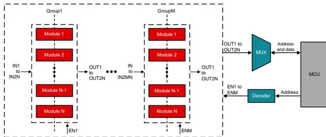
Figure 2. Block diagram of a DI board system
