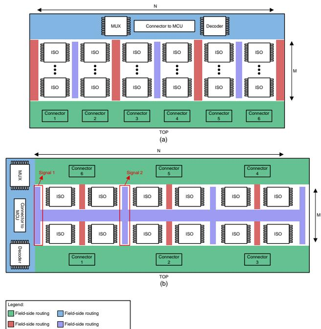
Figure 3. Two floor design solution for multi-channels digital input board design
