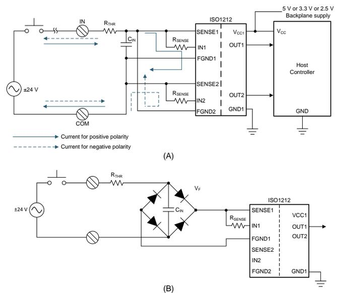
**Figure 1. Two solutions for bi-directional signal detection (a) ISO1212 with sourcing and sinking input (b) ISO1212 with Bridge rectifier**
