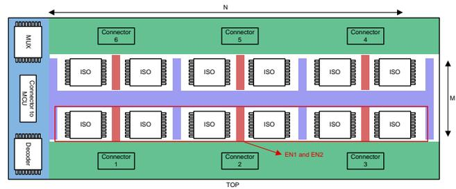
**Figure 5. Floor plan design of multi-channels DI board**
