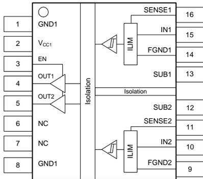
**Figure 4. Top view of ISO1212 DBQ Package**
