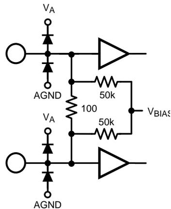
**Figure 14. RCLK Equivalent Circuit**
