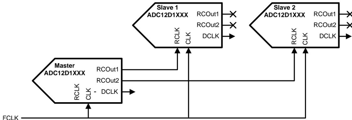
**Figure 1. Synchronizing Multiple ADCs Using AutoSync**
