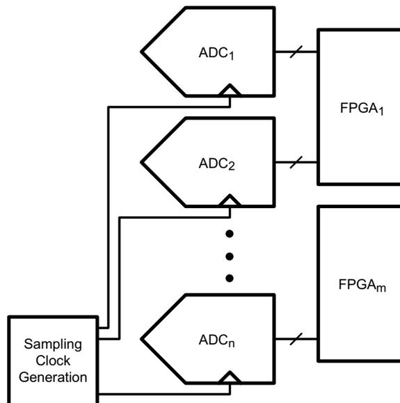
**Figure 2. Multiple ADCs in a System**
