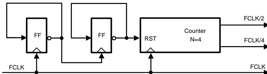
Figure 5. DCLK Generation for Master Mode
