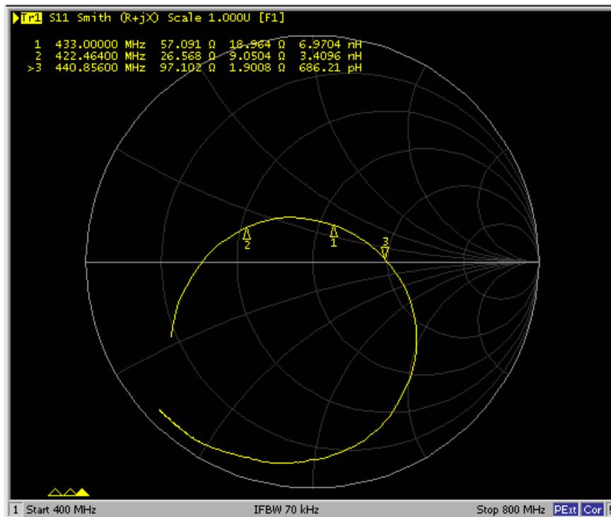
Figure 9. Matching of the Antenna With ANT1 and ANT2 Components
