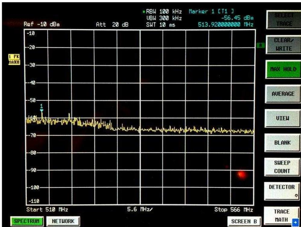
Figure 8. Conductive Spurious Emission on 510 MHz to 566 MHz
