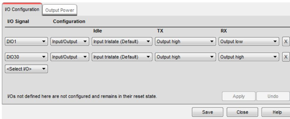
**Figure 5. DIO Configuration in SmartRF Studio 7**
