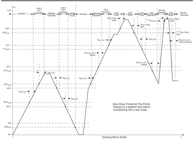
图 9-2. TS Battery Temperature Bias Threshold and Deglitch Timers
