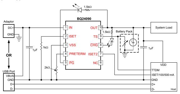
图 10-1. Typical Application Schematic
