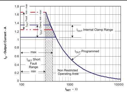
图 9-5. Programmed/Clamped Out Current
