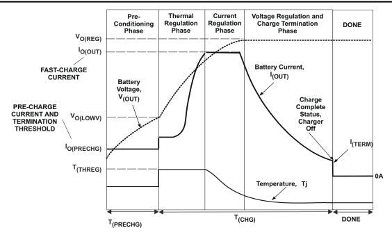
图 9-1. Charging Profile with Thermal Regulation
