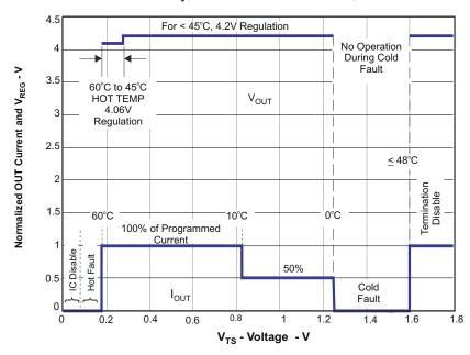
图 9-4. Operation Over TS Bias Voltage
