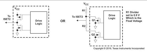
图 9-6. Configurations for Driving the 3-State ISET2 Pin
