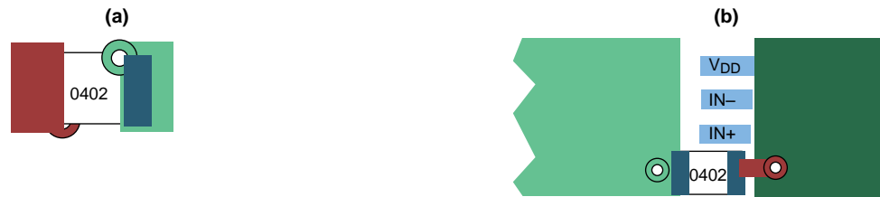
图 29. Typical Decoupling Capacitor Layouts
