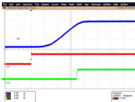
图 10-13. Dominant to Recessive Propagation Delay
