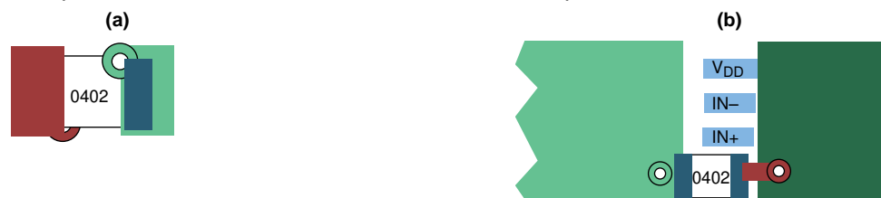
图 28. Typical Decoupling Capacitor Layouts
