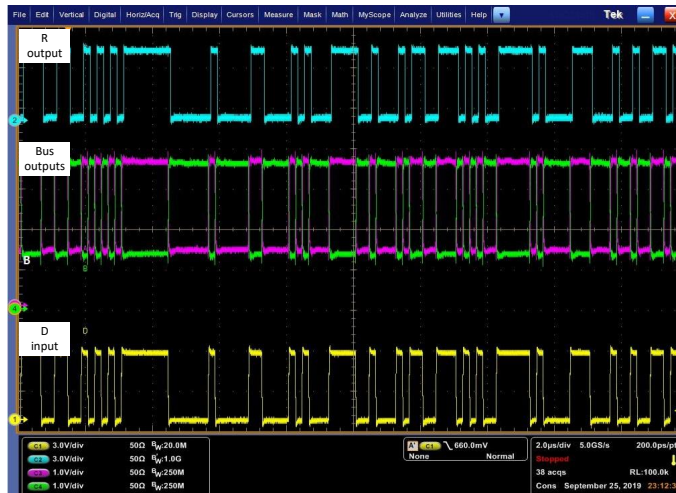
图 22. Waveforms at 10 Mbps Operation, PRBS7 Data Pattern
