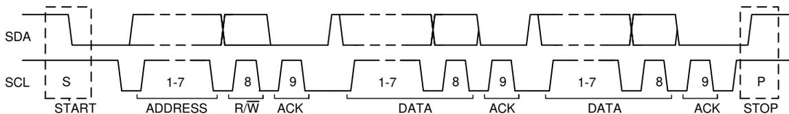
图 8-17. Complete Data Transfer on the I<sup>2</sup>C Bus
