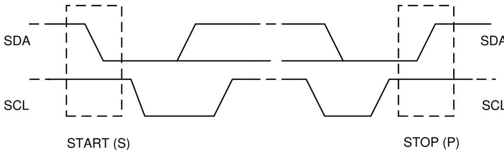
图 8-14. START and STOP Conditions on the I<sup>2</sup>C Bus
