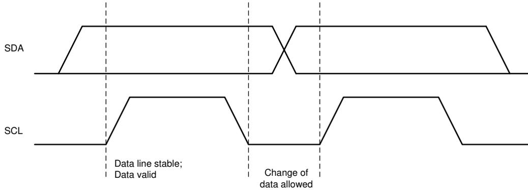
图 8-13. Bit Transfers on the I<sup>2</sup>C Bus
