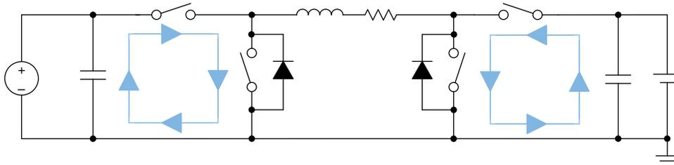
图 11-1. Buck-Boost Converter High Frequency Current Path
