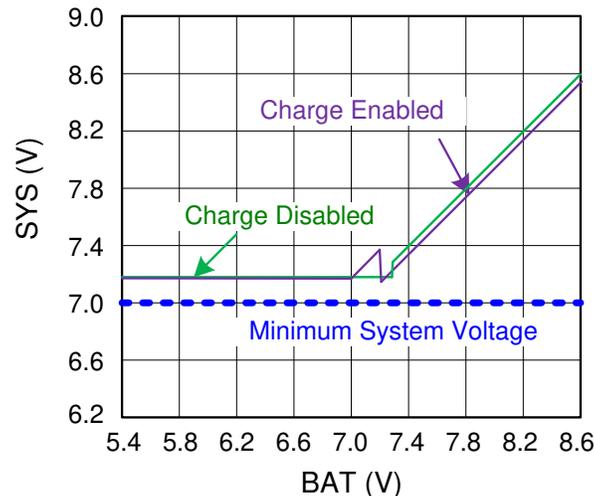
图 8-6. Typical System Voltage vs Battery Voltage for a 2S Battery Configuration
