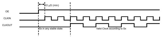
NOTE: Transition to new state will happen after a latency of 2 input clock cycles excluding the input cycle where the transition has occurred.
