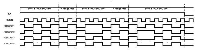
NOTE: Transition to new state will happen after a latency of one output clock cycle after completing the present output clock cycle. Transition to new state will happen after a latency of up to 3 input clock cycles excluding the input cycle where the transition has occurred.
