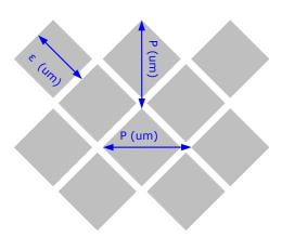
Figure 14. Mirror (Pixel) Pitch
