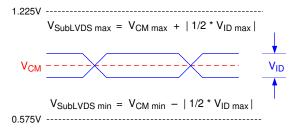
Figure 7. SubLVDS Waveform Parameters
