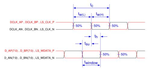
Figure 4. SubLVDS Switching Parameters
