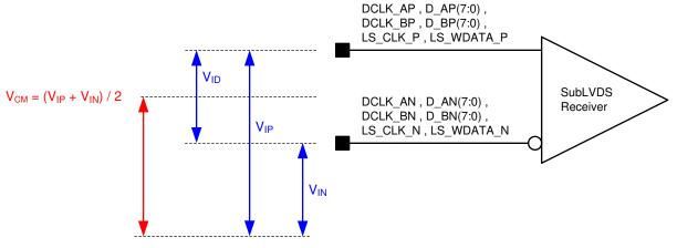
Figure 6. SubLVDS Voltage Parameters
