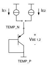
Figure 17. Temperature Measurement Theory
