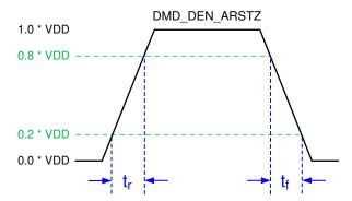
Figure 2. LPSDR Input Rise and Fall Slew Rate
