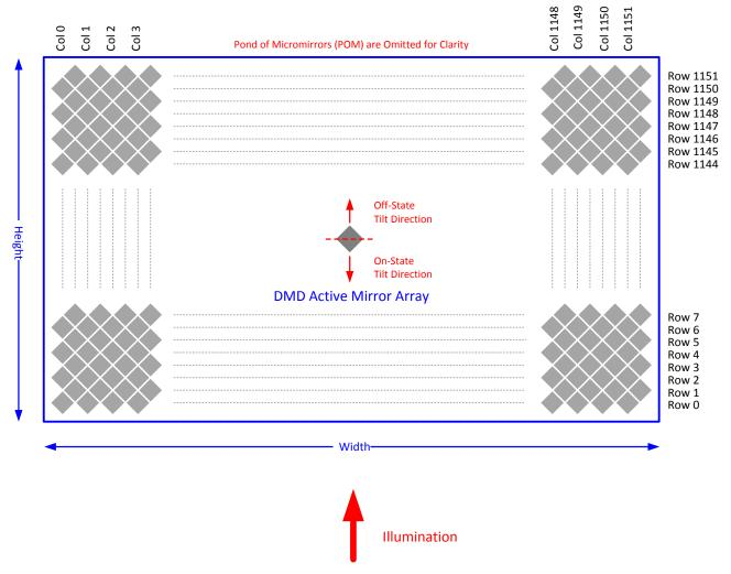
Figure 15. 0.55-in 1.3-MP Micromirror Array
