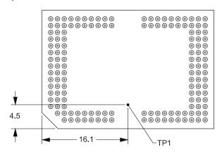
Figure 19. DMD Thermal Test Points
