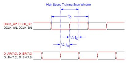
Figure 5. High-Speed Training Scan Window
