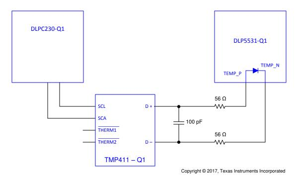
Figure 16. Temperature Sense Diode Typical Circuit Configuration
