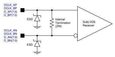
Figure 8. SubLVDS Equivalent Input Circuit
