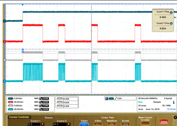
图 8-9. ITRIP Across TOFF and Load Current
