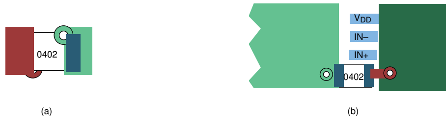
图 11-7. Typical Decoupling Capacitor Layouts
