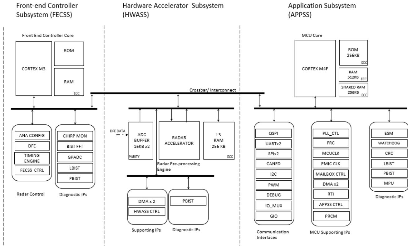
Figure 8-4. Processor Subsystem
