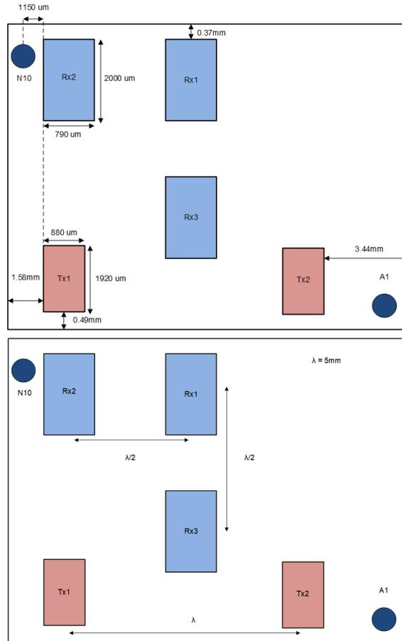
**Figure 7-9. Antenna Positions (Placement and Relative Spacing)**
