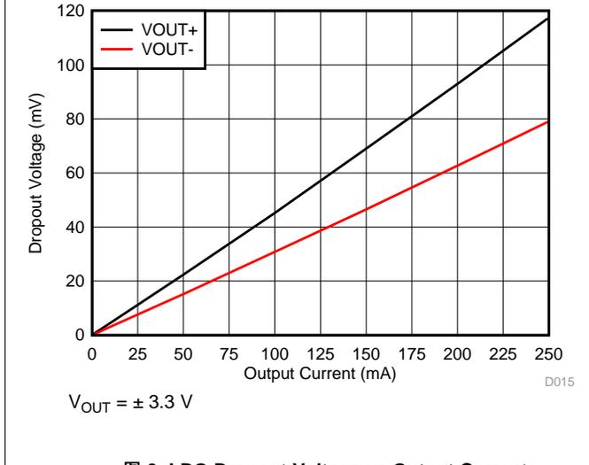
图 3. LDO Dropout Voltage vs Output Current
