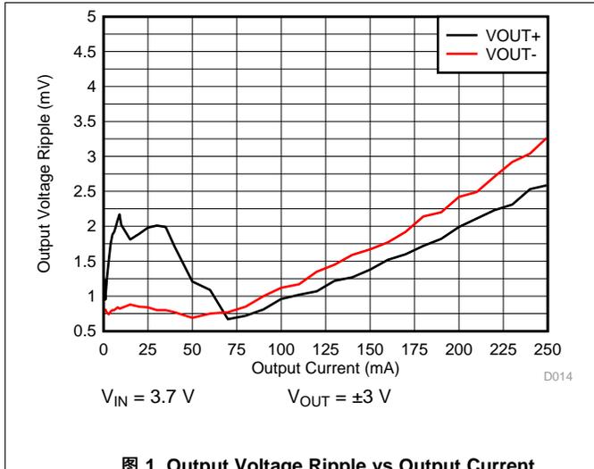
图 1. Output Voltage Ripple vs Output Current
