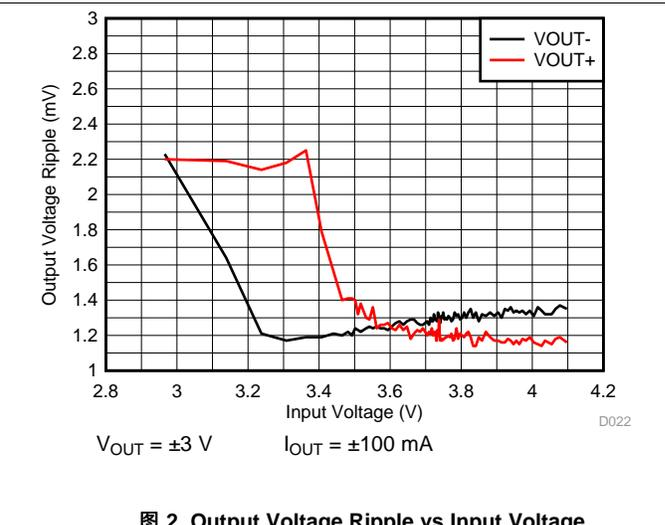
图 2. Output Voltage Ripple vs Input Voltage
