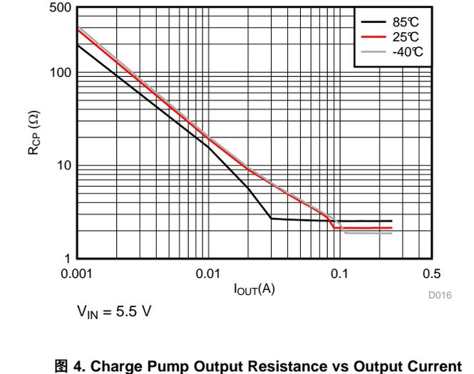
图 4. Charge Pump Output Resistance vs Output Current
