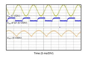
Figure 13. Response to 100Hz AC Input
