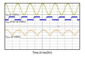
Figure 12. Response to 60Hz AC Input
