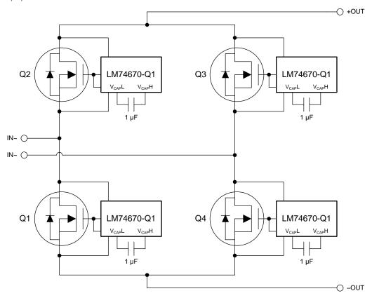
Figure 11. Typical Full Bridge Rectifier Application
