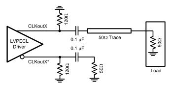
Figure 34. Single-Ended LVPECL Operation, AC-Coupling
