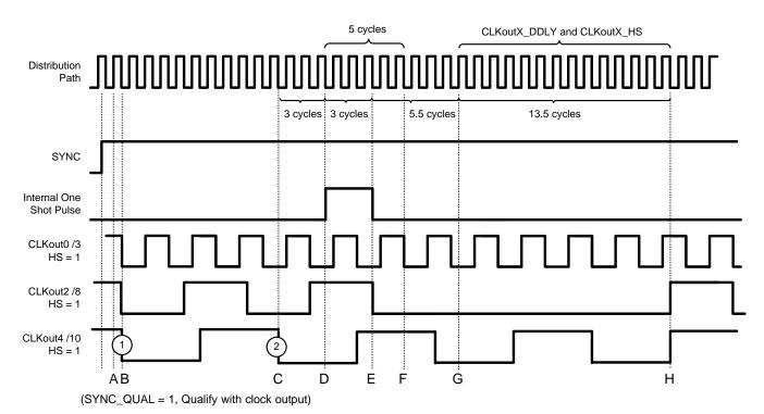
Figure 13. Absolute Dynamic Digital Delay Programming Example
