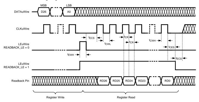
Figure 9. MICROWIRE Readback Timing Diagram
