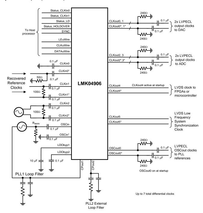
Figure 39. Example Application – System Schematic Except for Power
