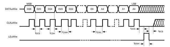
Figure 6. MICROWIRE Timing Diagram
