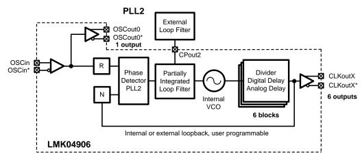
Figure 18. Simplified Functional Block Diagram for 0-delay Single Loop Mode
