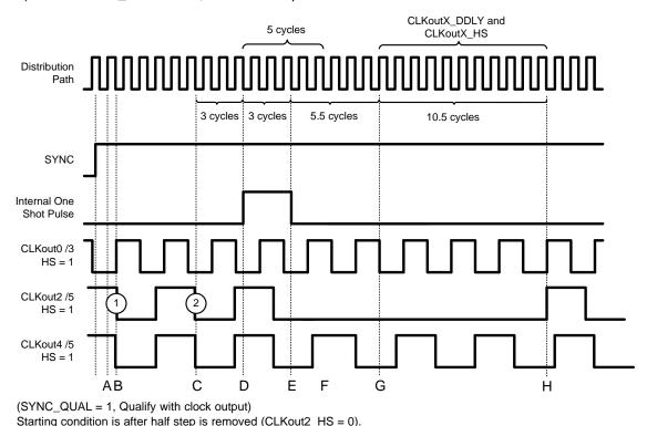
Figure 14. Relative Dynamic Digital Delay Programming Example—2nd Adjust
