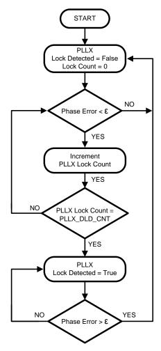
Figure 10. Digital Lock Detect Flowchart
