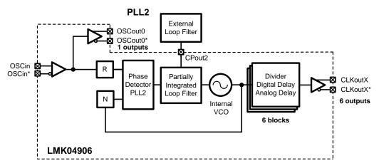
Figure 17. Simplified Functional Block Diagram for Single Loop Mode
