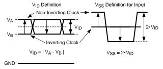
Figure 4. Two Different Definitions for Differential Input Signals
