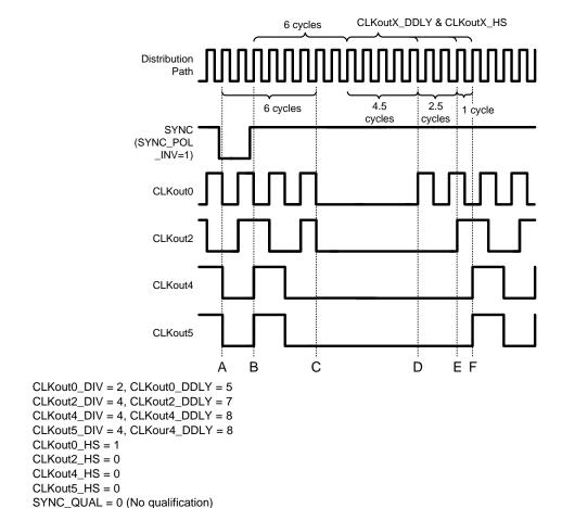
Figure 12. Clock Output Synchronization Using the SYNC Pin (Active Low)
