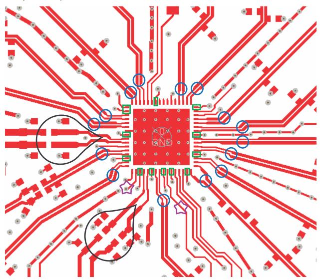
CLKin and OSCin path – if differential input (preferred) route trace tightly coupled like clock outputs. If single ended, have at least 3 trace width (of CLKin/OSCin trace) separation from other RF traces.
