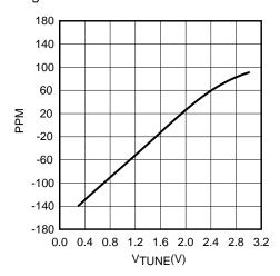
Figure 36. Example Tuning Curve, 20.48-MHz Crystal
