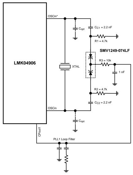
Figure 35. Reference Design Circuit for Crystal Oscillator Option
