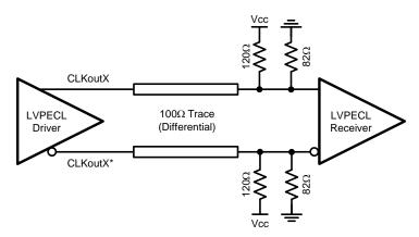
Figure 28. Differential LVPECL Operation, DC Coupling, Thevenin Equivalent
