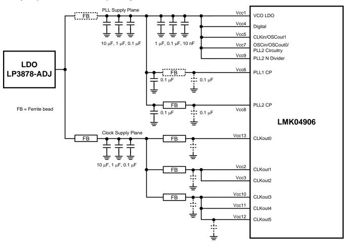
Figure 40. Example Application - Power System Schematic
