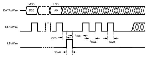
Figure 7. MICROWIRE Timing Diagram: Extra CLKuWire Pulses for R0 to R5
