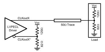
Figure 33. Single-Ended LVPECL Operation, DC Coupling, Thevenin Equivalent
