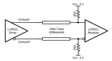
Figure 27. Differential LVPECL Operation, DC Coupling
