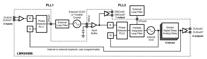
Figure 16. Simplified Functional Block Diagram for 0-delay Dual Loop Mode
