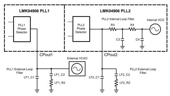
Figure 20. PLL1 and PLL2 Loop Filters
