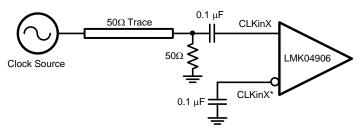
Figure 24. CLKinX/X\* Single-Ended Termination
