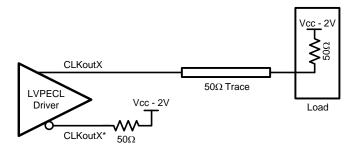
Figure 32. Single-Ended LVPECL Operation, DC Coupling
