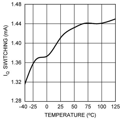
Figure 13. I<sub>Q</sub> Switching vs Temperature
