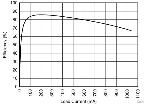
SN6505B + Würth 750316028 V_{CC} = 3.3\text{ V}
