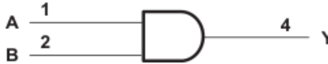
图 7-1. Logic Diagram (Positive Side)
