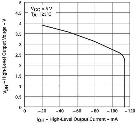
图 5-1. High-level Output Voltage vs High-level Output Current
