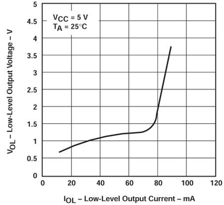
图 5-2. Low-level Output Voltage vs Low-level Output Current
