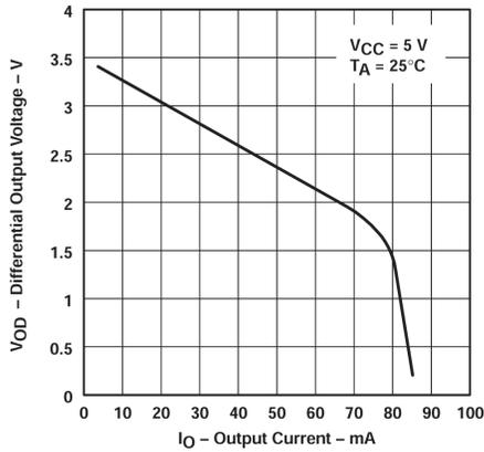
图 5-3. Differential Output Voltage vs Output Current
