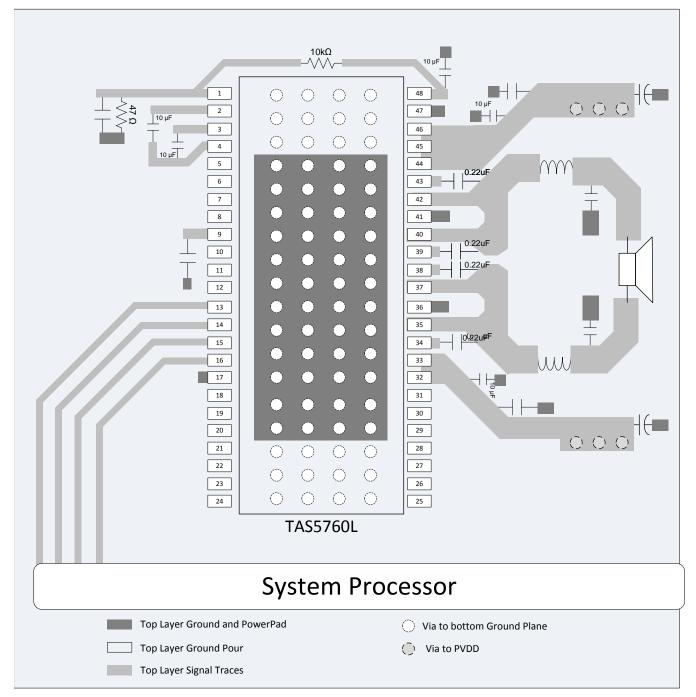
Figure 67. DCA Package PBTL Configuration
