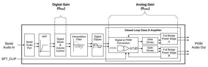
Figure 43. Speaker Amplifier Gain Structure
