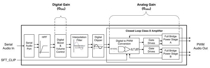
Figure 38. Speaker Amplifier Audio Signal Path
