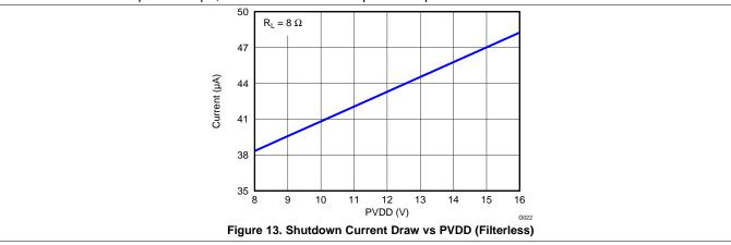
At  $T_A = 25^{\circ}$ C,  $f_{SPK\_AMP} = 768$  kHz, input signal is 1 kHz Sine, unless otherwise noted. Filter used for 8  $\Omega = 22 \mu$ H + 0.68  $\mu$ F, Filter used for 6  $\Omega = 15 \mu$ H + 0.68  $\mu$ F, Filter used for 4  $\Omega = 10 \mu$ H + 0.68  $\mu$ F unless otherwise noted.
