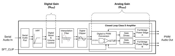
Figure 42. Speaker Amplifier Gain Select (SPK\_GAIN [1:0] Pins)
