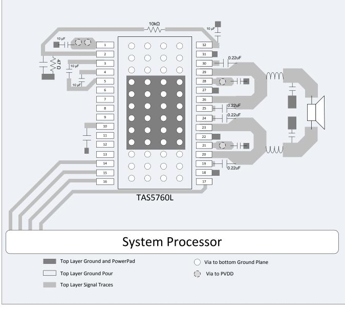
Figure 65. DAP Package PBTL Configuration
