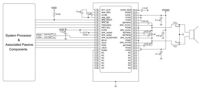
Figure 59. Mono PBTL Using Software Control
