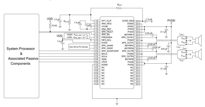
Figure 58. Stereo BTL Using Hardware Control
