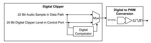
Figure 39. Digital Clipper Simplified Block Diagram
