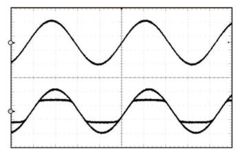
Figure 41. Soft Clipper Example Wave Form
