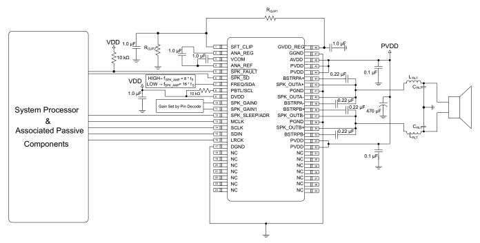
Figure 60. Mono PBTL Using Hardware Control
