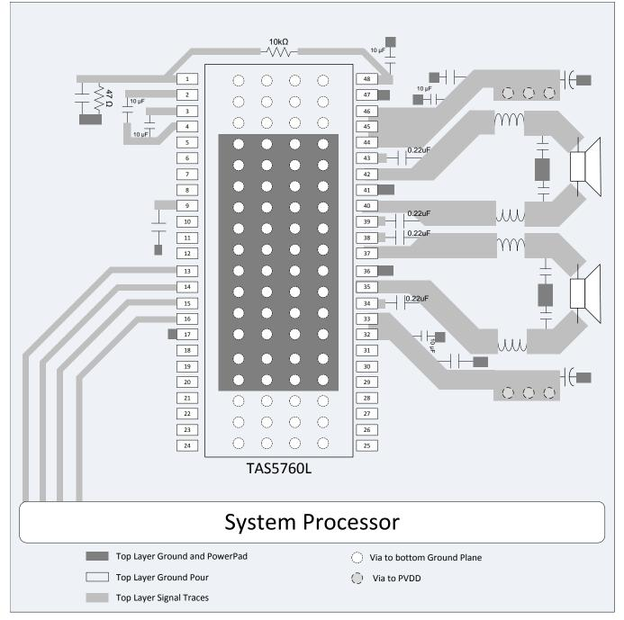
Figure 68. DCA Package BTL Configuration
