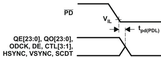
图 8-7. Delay From PD Low to Hi-Z Outputs
