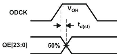
图 8-5. ODCK High to QE[23:0] Staggered Data Output
