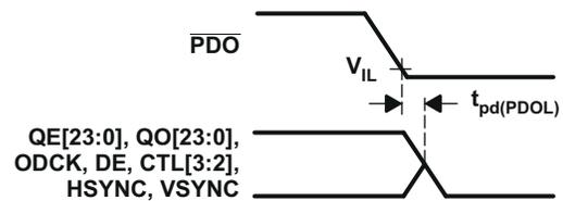
图 8-8. Delay From PDO Low to Hi-Z Outputs
