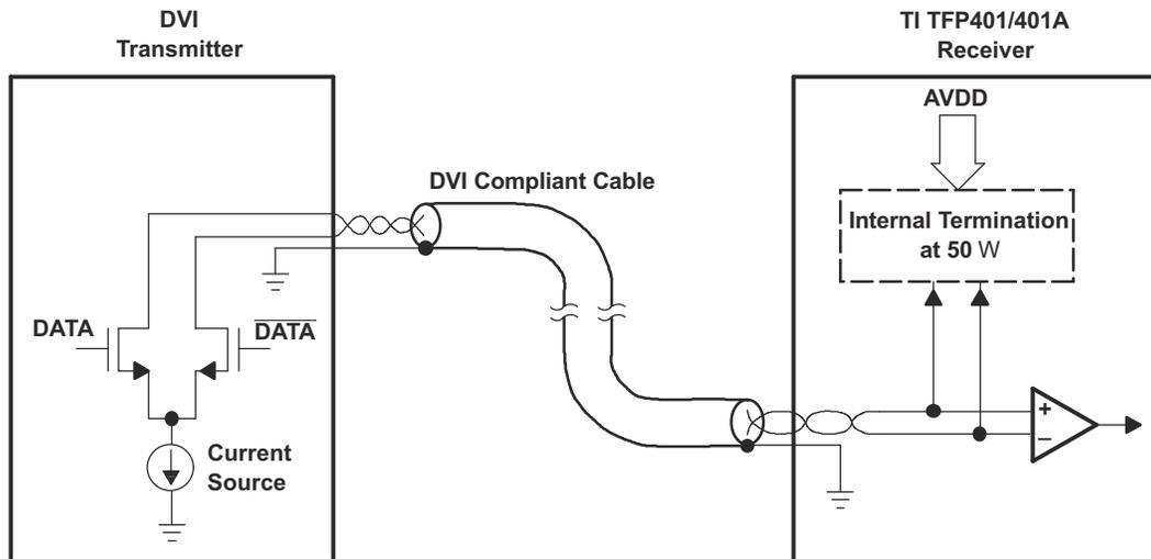
图 9-1. TMDS Differential Input and Transmitter Connection
