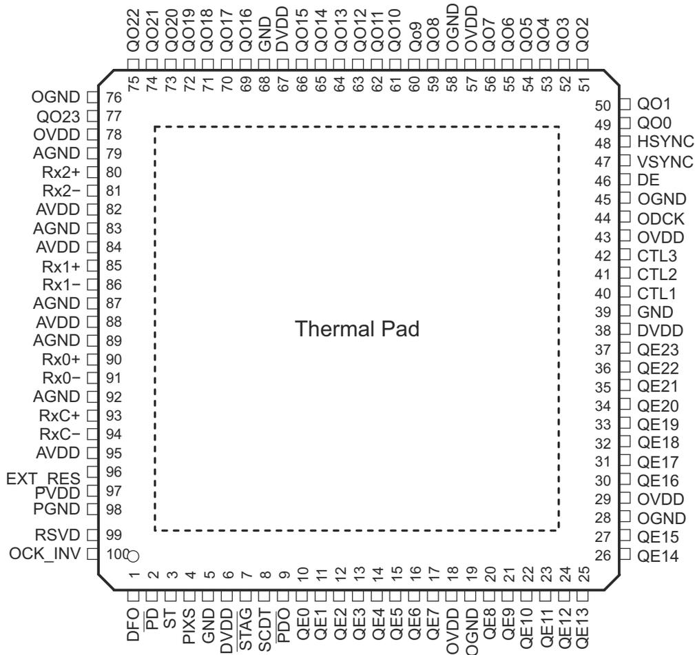
图 6-1. PZP Package, 100-Pin HTQFP (Top View)
