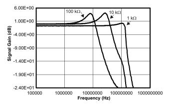
Figure 38. THS4521 Frequency Response with Various Gain Setting and Load Resistor Values
