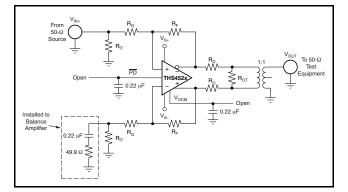
Figure 28. Distortion Test Circuit
