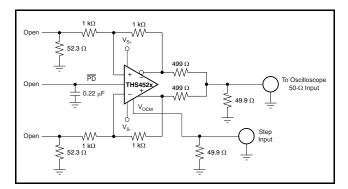
Figure 33. V<sub>OCM</sub> Transient Response and Slew Rate Test Circuit
