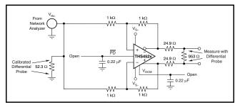
Figure 30. CMRR Test Circuit
