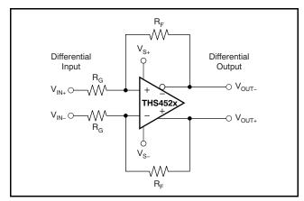
Figure 34. Differential Input to Differential Output Amplifier
