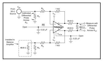
Figure 27. Frequency Response Test Circuit
