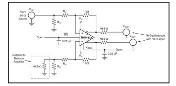
Figure 29. Slew Rate, Transient Response, Settling Time, Output Impedance, Overdrive Recovery, V<sub>OUT</sub> Swing, and Turn-On/Turn-Off Test Circuit
