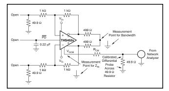
Figure 32. V<sub>OCM</sub> Input Test Circuit
