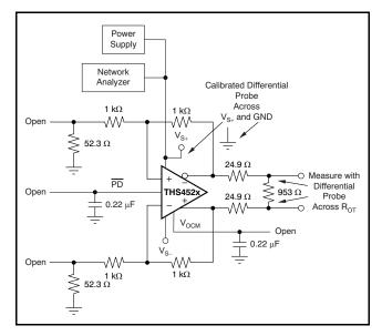
Figure 31. PSRR Test Circuit
