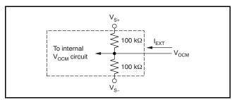
Figure 36. V<sub>OCM</sub> Input Circuit
