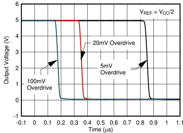
图 6-34. Response Time for Various Overdrives, High-to-Low Transition
