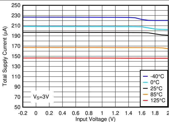
图 6-5. Total Supply Current vs. Input Voltage at 3V
