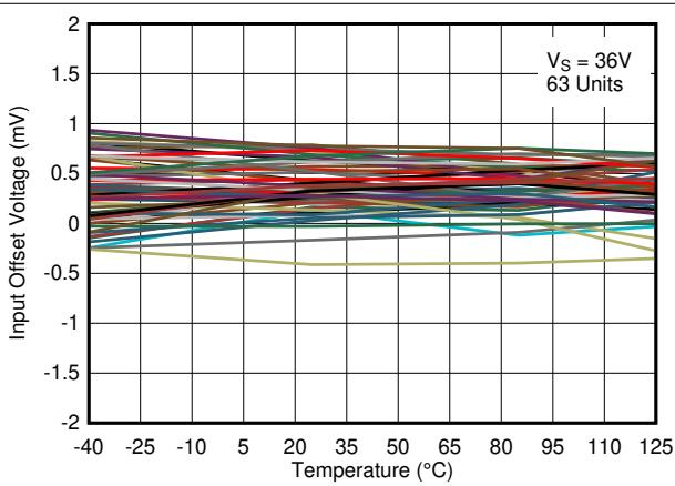
图 6-21. Input Offset Voltage vs. Temperature at 36V
