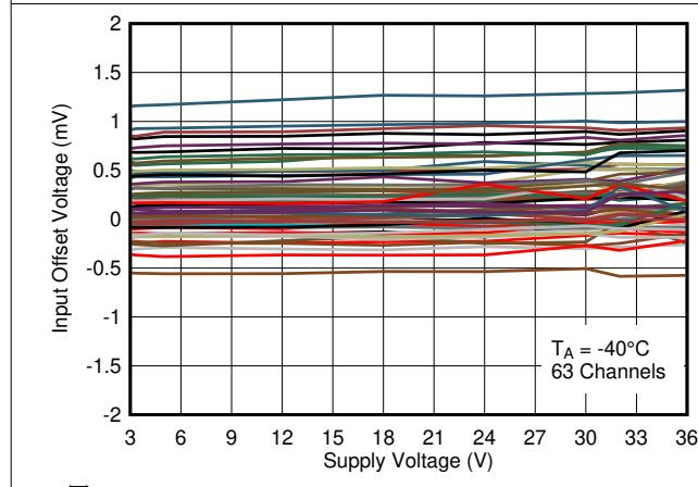
图 6-14. Input Offset Voltage vs. Supply Voltage at -40°C
