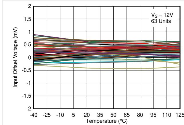
图 6-20. Input Offset Voltage vs. Temperature at 12V
