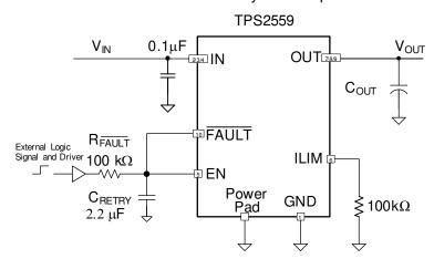
图 9-4. Auto-Retry Circuit with External EN Signal
