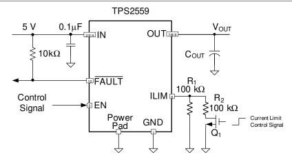
图 9-5. Two-Level Current-Limit Circuit
