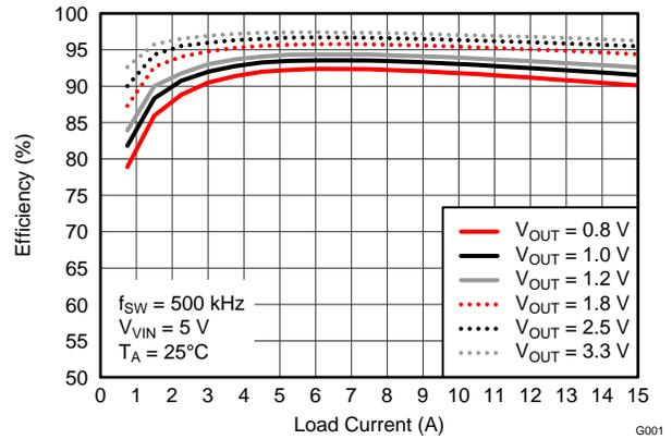
Figure 16. Efficiency vs. Load Current ( $V_{VIN} = 5 V$ )
