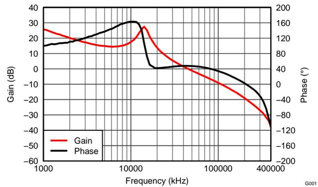
Figure 22. Loop Response, 47-kHz Bandwidth, 48° Phase Margin
