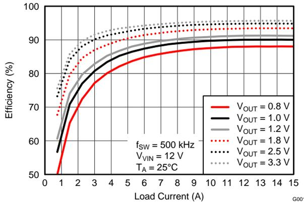
Figure 15. Efficiency vs. Load Current ( $V_{VIN} = 12 V$ )
