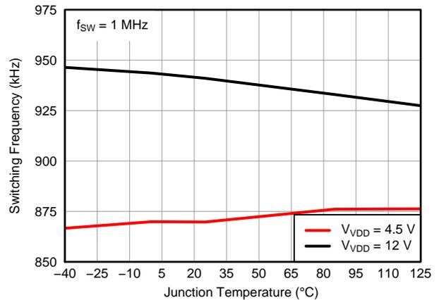
Figure 4. Switching Frequency vs. Junction Temperature (1 MHz)
