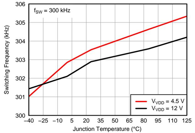
Figure 2. Switching Frequency vs. Junction Temperature (300 kHz)
