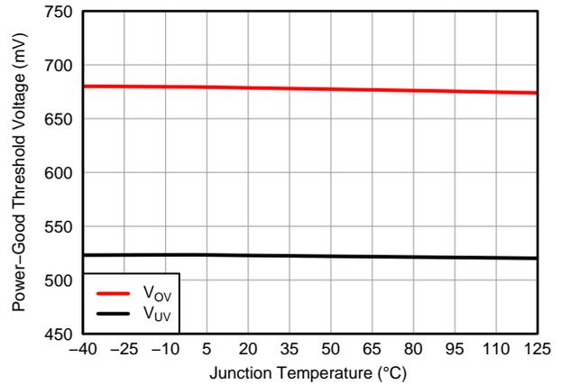
Figure 14. Power Good Threshold Voltage vs. Junction Temperature
