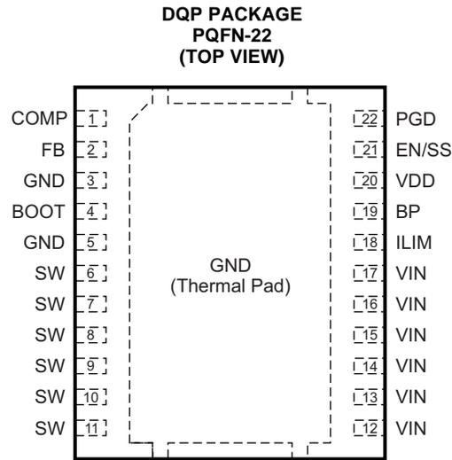
Note: The thermal pad is also an electrical ground connection.
