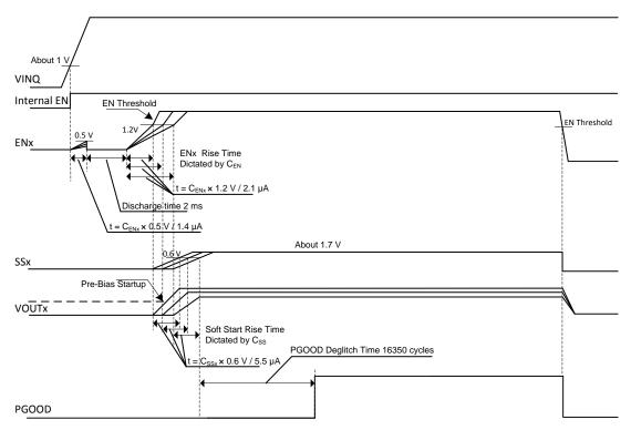
Figure 27. Startup Power Sequence
