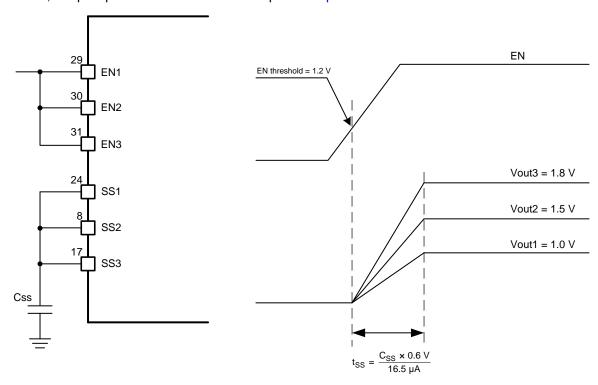
Figure 25. Ratiometric Power-Up Using SSx Pins
