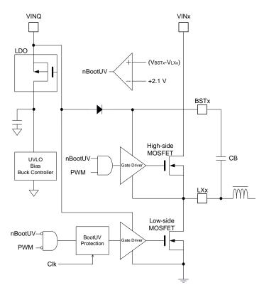
Figure 28. Bootstrap Voltage and Diagram
