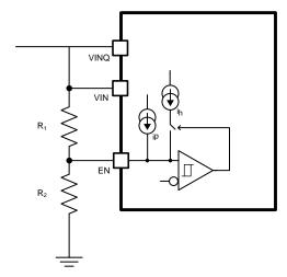
Figure 24. Adjustable VIN and VINQ UVLO
