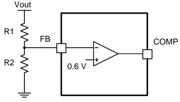
Figure 21. Voltage Divider Circuit
