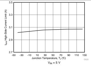
Figure 19. Buck2 High-Side Current Limit vs Temperature
