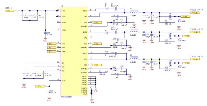
Figure 32. Typical Application Schematic
