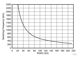
Figure 30. ROSC vs Switching Frequency
