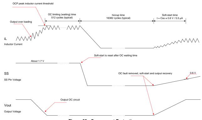
Figure 29. Overcurrent Protection
